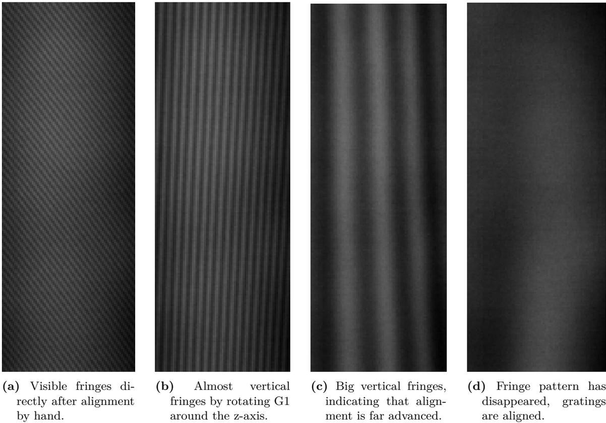
**Fig. 3.3.:** Grating alignment flow. The slight divergence towards the bottom seen in Fig. 3.3c can be corrected by rotating G1 around the  $x$ -axis.
