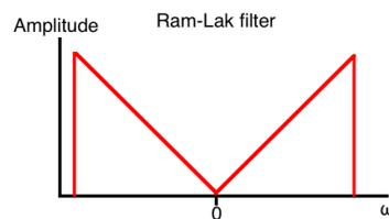
**Fig. 2.5.:** Ram-Lak filter that attenuates low spatial frequencies (around  $\omega = 0$ ) and lets high spatial frequencies pass [1]. This filter counteracts the underrepresentation of high spatial frequencies when using reconstruction algorithms that are based on the Fourier slice theorem.
