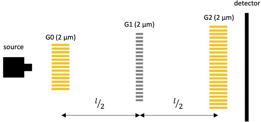
**Fig. 2.1.:** Symmetric setup with gold filled absorption gratings and  $\pi$  shifting phase grating. Sample placement is between  $G_0$  and  $G_1$
