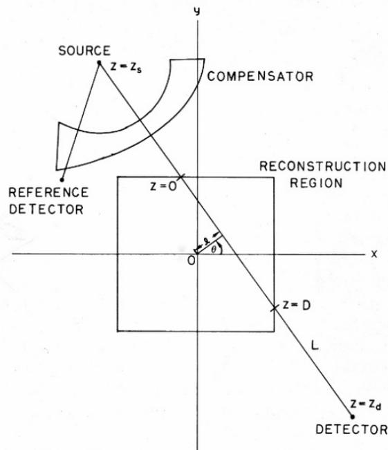
**Fig. 2.2.:** Computerized Tomography acquisition protocol [7, p. 30].  $\theta$  is the angle at which the acquisition happens,  $l$  the deviation to the side. The detector measures the intensity of the attenuated beam and together with a flat-field measurement, the attenuation  $A$  can be derived.
