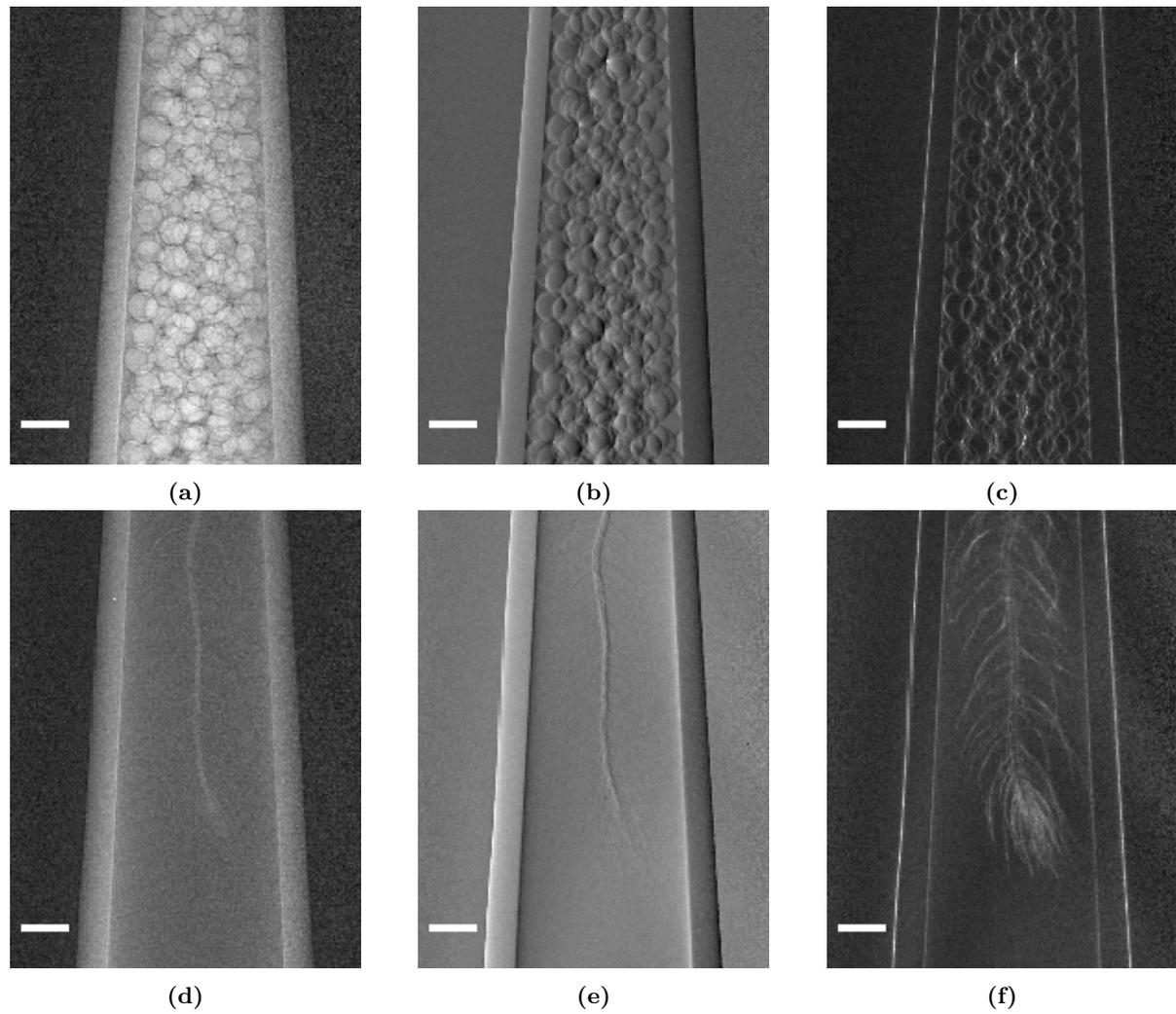
**Fig. A.3.:** Absorption (a, d), differential phase (b, e) and dark field (c, f) contrast images of two samples - polystyrene balls of 700  $\mu\text{m}$  and stem of Poaceae, respectively. The plant (Poaceae) sample is almost transparent in the absorption and phase contrast regimes, while the dark-field image clearly reveals more details of its inner structure. Scale bars at all images corresponds to 1 mm at the sample position as the magnification factor of 2 is taken into account.
