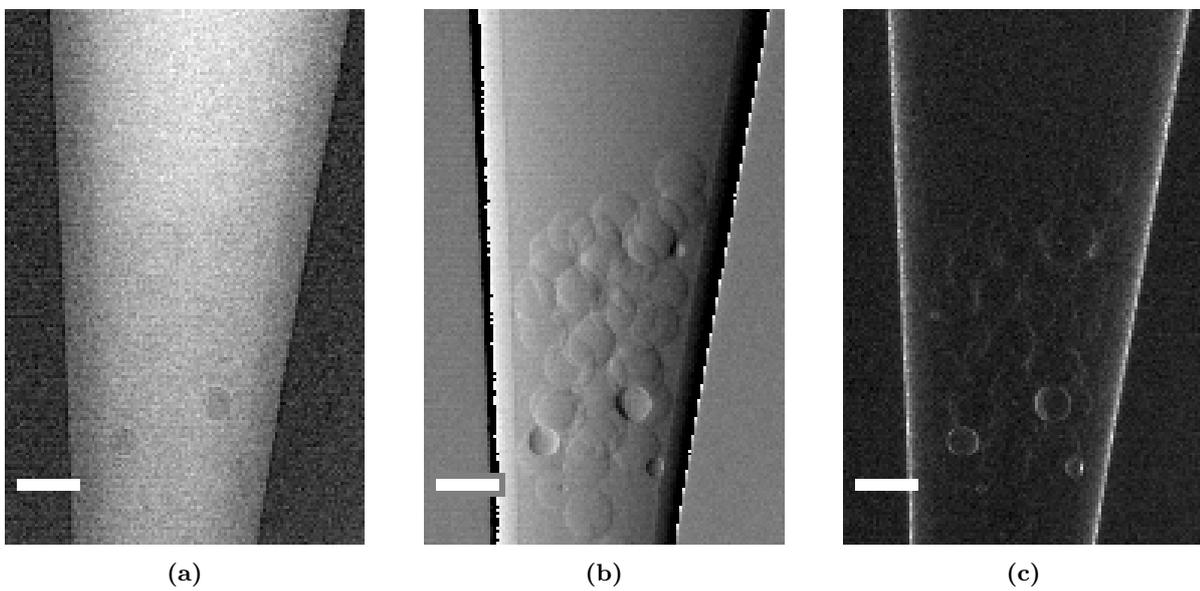
**Fig. A.4.:** Absorption (a), differential phase (b) and dark field (c) contrast images of the polystyrene balls with the diameter of  $700\ \mu\text{m}$  placed in the ethanol. The sample provides no contrast in the absorption mode while clearly revealing its structure in the differential phase image and, partially, - in the dark field image. Scale bars at all images corresponds to 1 mm at the sample position as the magnification factor of 1.6 is taken into account.
