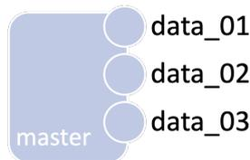
**Fig. 4.2.:** File structure of *Eiger's HDF5* files.
