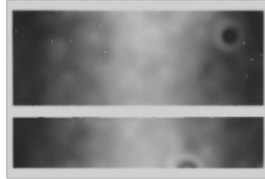
(b) The transmission profile of a  $2\ \mu\text{m}$  grating. Apart from some inhomogeneities in the right part (circles), it can be seen that transmission is higher in the center part.
