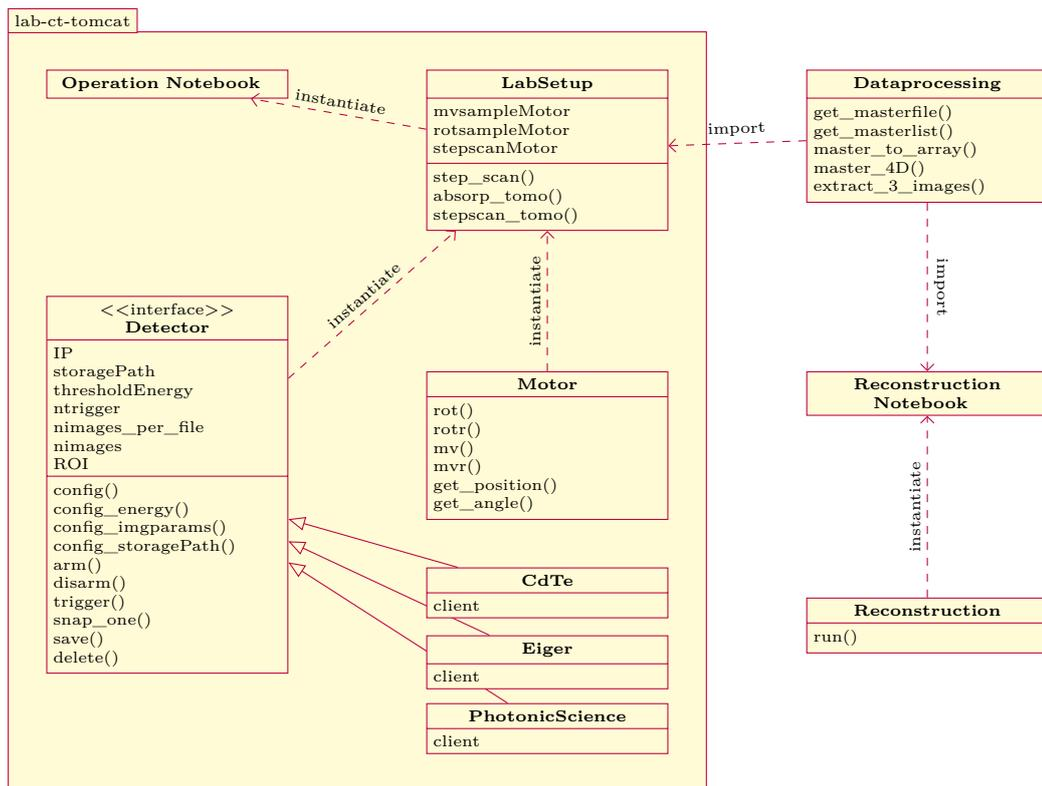
**Fig. 4.1.:** Class Chart. The interface `Detector` defines the functions and attributes that each detector should implement. `LabSetup` gets assigned 3 motors, a detector of a certain type and implements different functions that make use of all setup hardware. `Reconstruction` handles geometries and algorithms of the ASTRA toolbox. High-level operation happens in Jupyter Notebooks.
