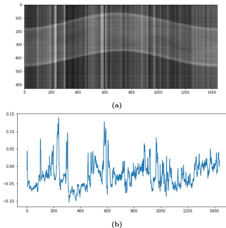
**Fig. 5.2.:** The figure in (a) shows a sinogram from a tomography with the Sigray source and murine lung sample. A total of 1440 projections was acquired (horizontal axis) over a time frame of 11 hours and after performing flat field correction with the same flat field for all projections the drift of the source was realized. The mean values of the lowest 100 pixels are shown in (b), indicating that the drift is very strong in the first 6 hours and gets better over time.
