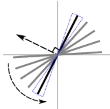
**Fig. 2.3.:** Fourier slice theorem. Shown is the 1D Fourier transform of the projections (gray and black lines) in the 2D Fourier space. A 2D back transformation would yield the sample space, but the undersampling in the outer regions is well visible (blue) [13].
