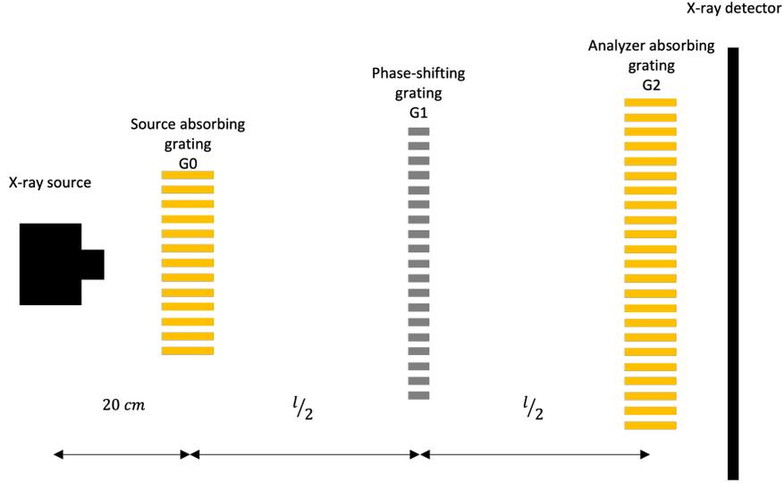
**Fig. A.1.:** A schematic of the symmetric X-ray grating interferometry setup, used for the quality assessment of the 1D gratings. Source- $G_0$  distance was 20 cm, and the detector was placed right behind  $G_2$ . For the case of the Talbot order 9, which was used for visibility measurements, the overall length  $l$  was 29 cm. For the case of the Talbot order 23, the overall length was 73.6 cm.
