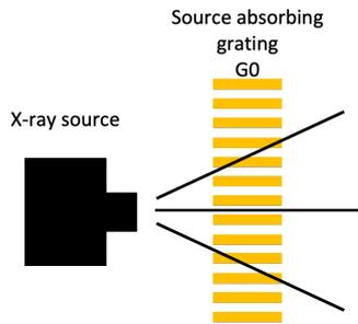
(a) The diverging beam of the X-ray source causes absorption in the outer parts of the grating. This limits the field of view.
