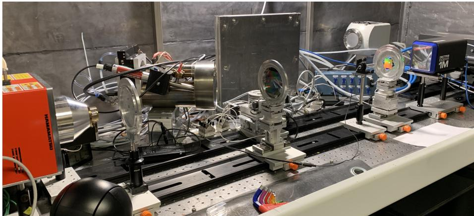
**Fig. 3.1.:** The setup as it was used during the course of this thesis. On the right the Dectris Eiger R 1M detector, the Hamamatsu L10101 microfocus source on the left and the three gratings on their respective motor towers in between on the rail.
