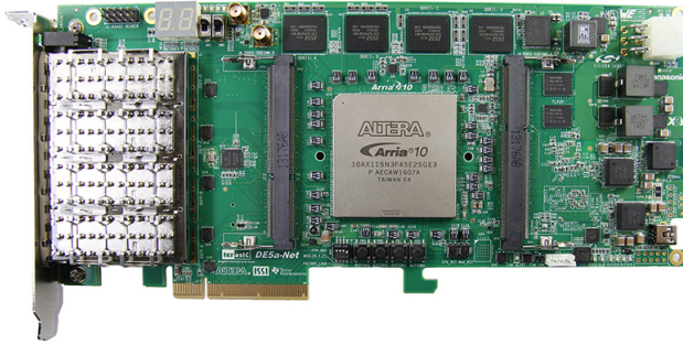
Figure 17.5: The DE5a NET board built by Terasic Inc. and used as a receiving board in the filter farm PCs. The Arria 10 FPGA with a PCIe Gen3 8 lane interface is complemented by a 16 duplex fast optical links and several GB of DDR4 memory.
