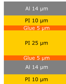
Figure 7.11: Stack chosen for the LTU produced 2-layer HDI circuits. PI=polyimide, Al=aluminium.
