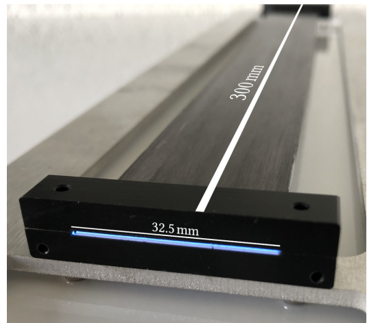
Figure 10.2: Full size SciFi ribbon prototype with preliminary holding structure. The SciFi ribbon is formed by staggering three layers of round scintillating fibres.
