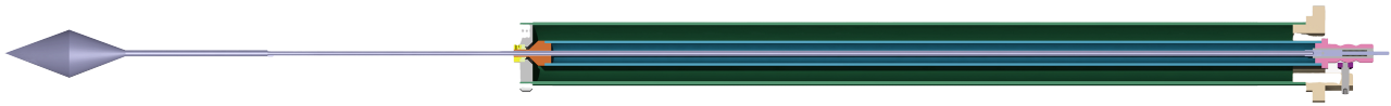
Figure 6.4: Cross section of target support and alignment mechanism. Muons hit the target from the left. The stopping target is mounted on a thin carbon tube which is steered and fixed in the support structure. The rear end of the support structure consists of an alignment mechanism to adjust the position of the target.
