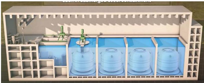
The study will address the natural convection heat transfer ( $HT$ ) from the external wall of the containment to the water pool for various conditions, including boiling of the pool
