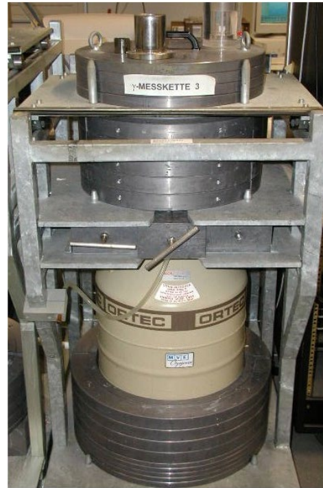
Laboratory: HPGe-Detector with shielding
