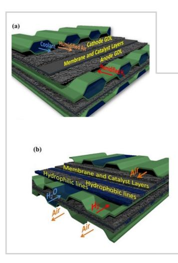
stream. To avoid accumulating water droplets in the GDL's small pores, which would block the pathways of the gases to the CL, the GDL is coated with a highly hydrophobic solution (very often, PTFE).
