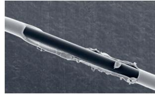
Open coating bicomponent fiber.
