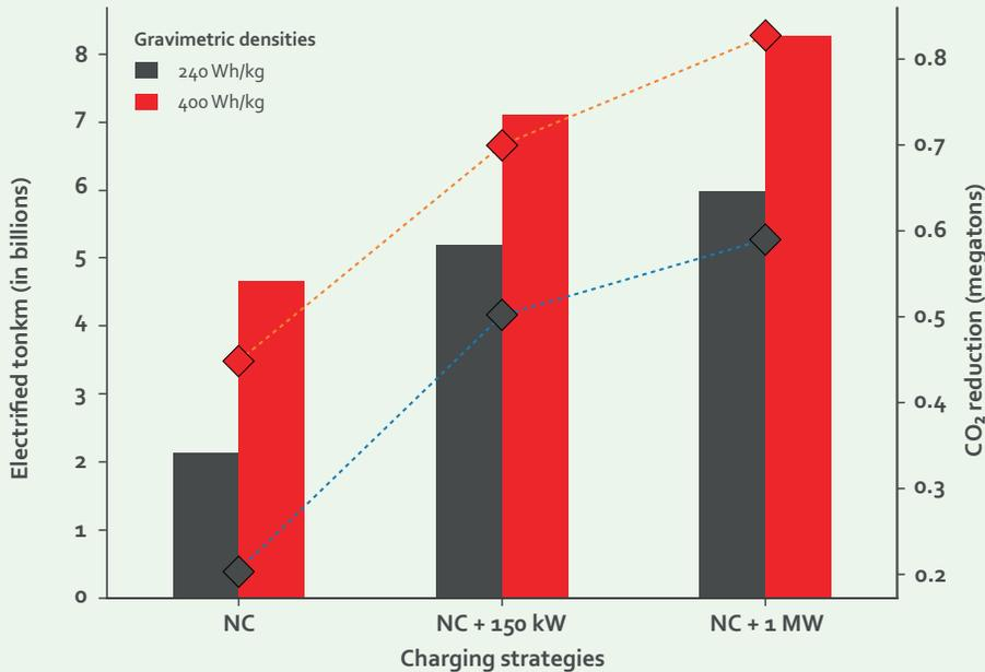
Number of ton kilometers (tonkm) that could be covered by battery electric trucks given different energy densities of batteries and charging strategies, along with CO<sub>2</sub> emissions avoided.
