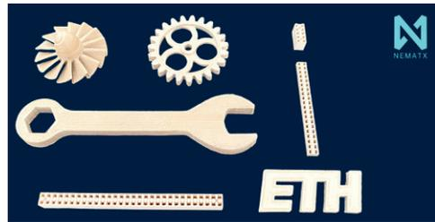
*Fully functional LCP objects fabricated with the nematic 3D printing technology.*
