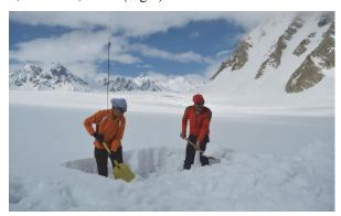
**Fig. 1:** Excavation of snow pits during the field survey at Biafo-Hispar glacier system in June/July 2019.
