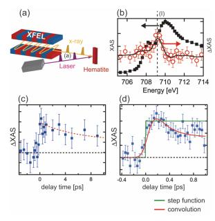
**Fig. 1:** pump probe XAS of hematite : (a) an illustration of the pump probe experiments in Pohang Accelerator Laboratory (PAL-XFEL) (b) Fe L<sub>3</sub> XAS of hematite (black) and difference XAS at a delaytime of 0.2 ps (red) (c) a kinetic trace at the energy point of 709 eV (denoted as (I) in (b) (d) a kinetic trace at the energy point of 709 eV around the vicinity of 0 ps.<sup>[4]</sup>
