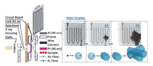
**Fig. 1:** Sketch of experimental setup is shown on the left (not to scale). The tilted optical microscope image of the Pt wire is shown. Three X-ray images on the right show water formation and the first instance of ice crystal formation followed by crystal growth.
