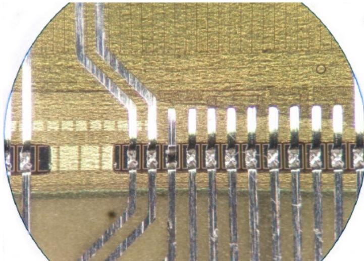
Operate MuPix on an aluminium-kapton flexprint without decoupling capacitors
