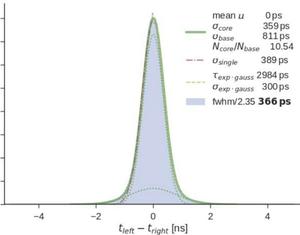
Timing resolution  $< 400\text{ ps}$  including ASIC
