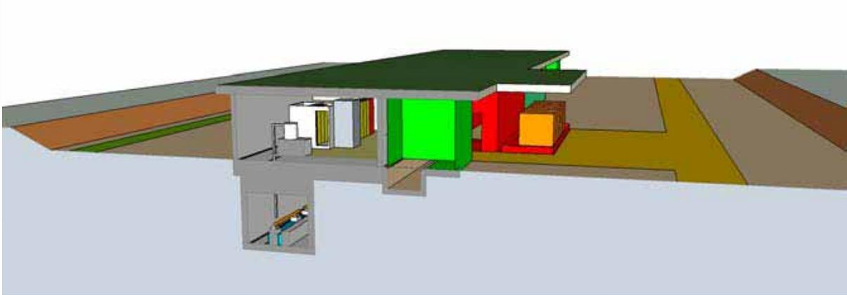
Fig. M.8. Cross-section of the accelerator, with the underground accelerator tunnel and the above-ground building for the RF-power supplies.
