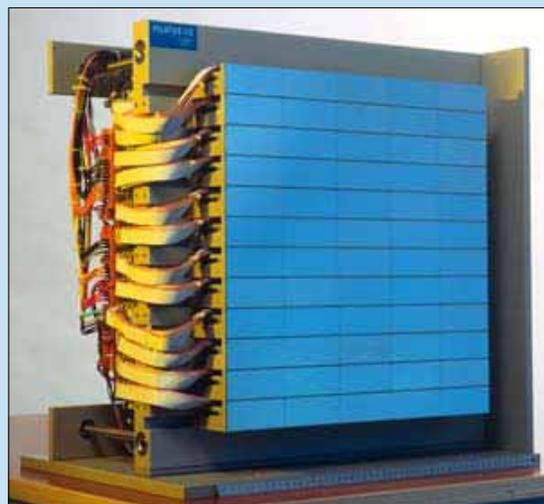
Fig. III.i6. The PILATUS 6M, with 6 million pixels, has been developed at PSI and commercialized by Dectris [31], a spin-off company from PSI, for applications in synchrotron-based protein crystallography.
