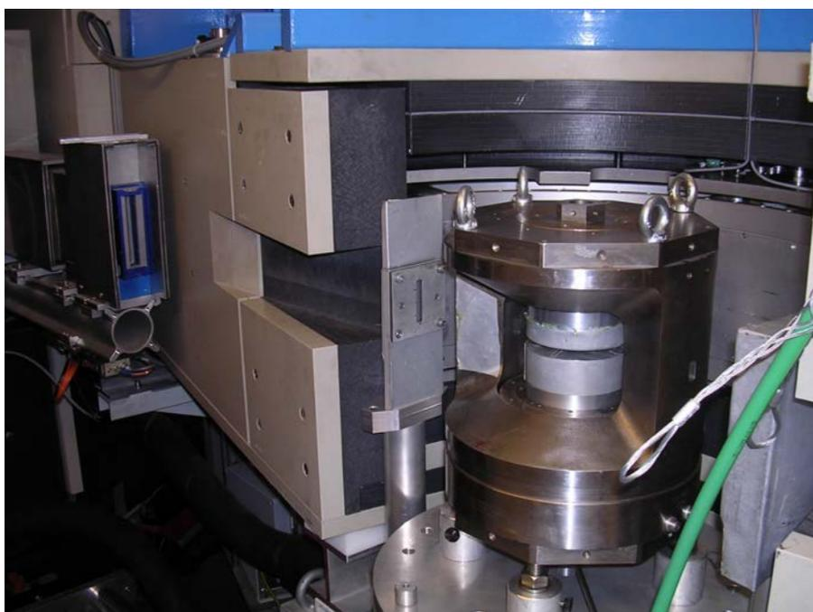
detector shielding + radial collimator + BN anvils + low noise electronics = excellent peak to background ratio
