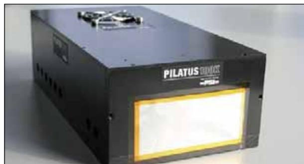
**The PILATUS 100K detector box. The active area of the detector is 84 x 34 mm<sup>2</sup>.**
