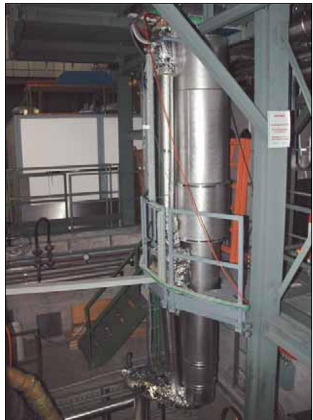
Figure 1: **View of the target in the test facility. The target is thermally insulated and equipped with a small bypass flow calibration loop at the bottom.**
