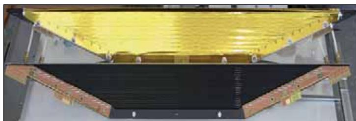
Figure 3: **First completed drift chamber module, showing inner anodes/cathodes and hood module (top).**
