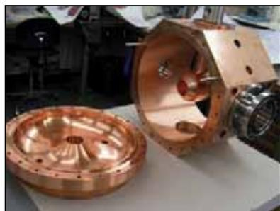
Figure 3: Components of the 500 MHz buncher to be installed in the 72 MeV beam transfer line to the ring cyclotron.
