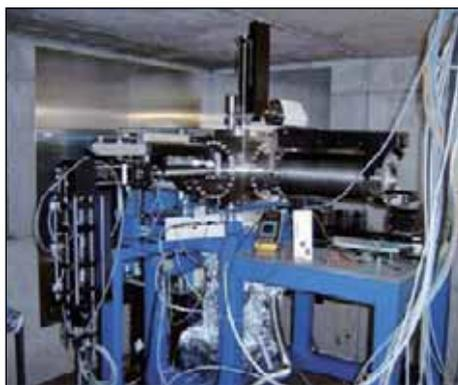
Figure 3: **100 kV DC test setup for first beam-diagnostics of field emitters: current, transverse profile and emittance.**
