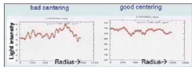
Figure 2: Light intensity on the radial probe, as a function of radius.
