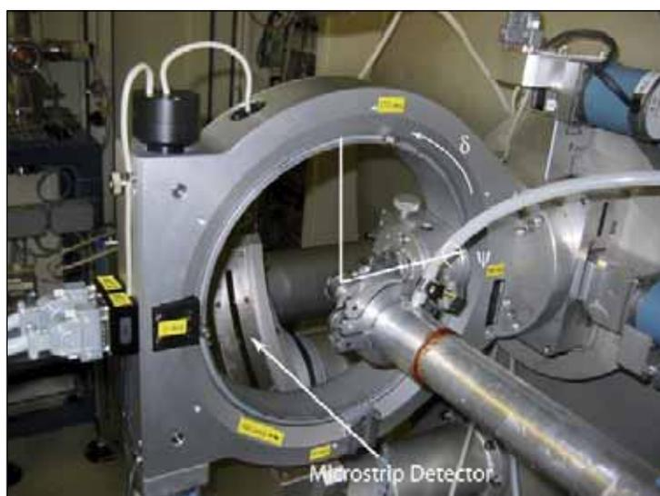
Figure 1: Experimental setup showing (1) the Eulerian cradle (angles  $\delta$  and  $\psi$ ) for orienting the sample in the beam, and (2) the Si-microstrip detector.
