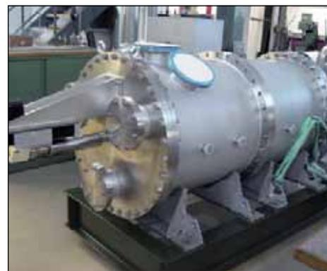
Figure 4: **High voltage tank of the 200 ns, 500 kV pulser.** The machining is designed as a test-environment that feeds pulses to a cathode and also permits a fast replacement of them in the case of electrical breakdowns.
