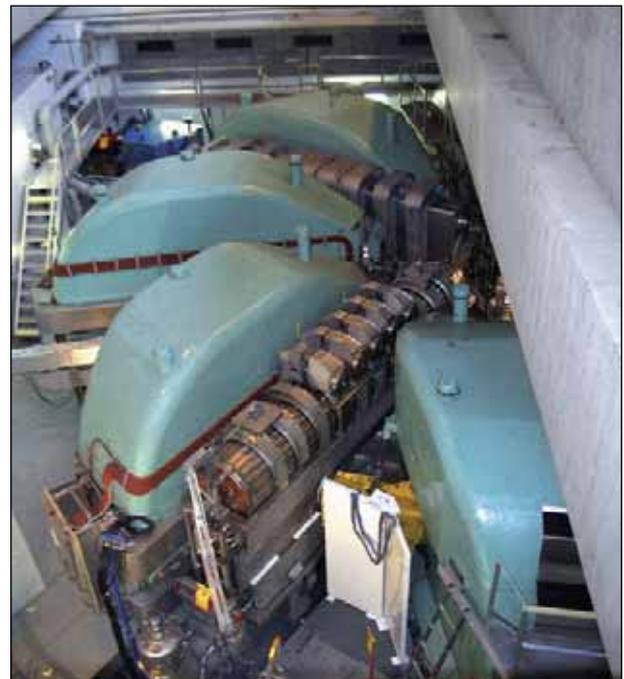
Figure 1: **Installation of the first new copper rf-cavity in the ring cyclotron.**
