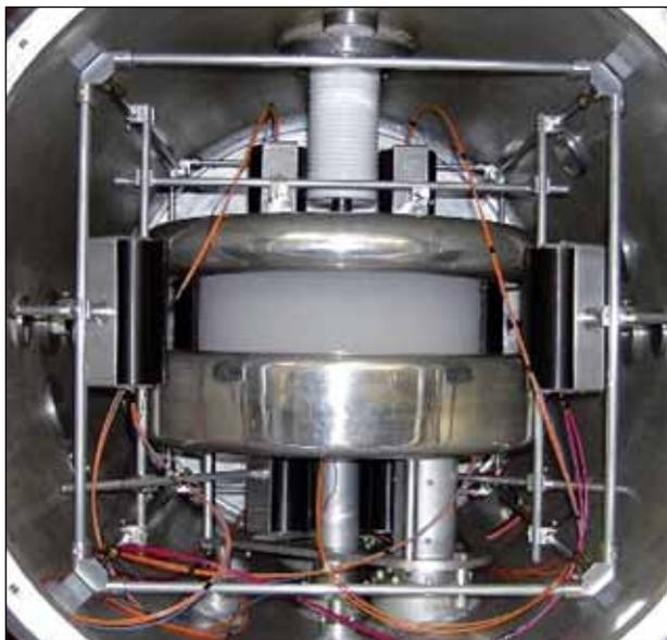
Figure 2: The inside of the EDM vacuum chamber showing the newly installed 8 CsM (black cylinders).
