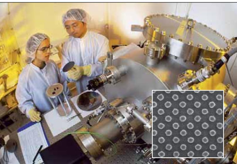
Figure 1: Exposure system at the XIL beamline. Inset shows a 50 nm period dot pattern.
