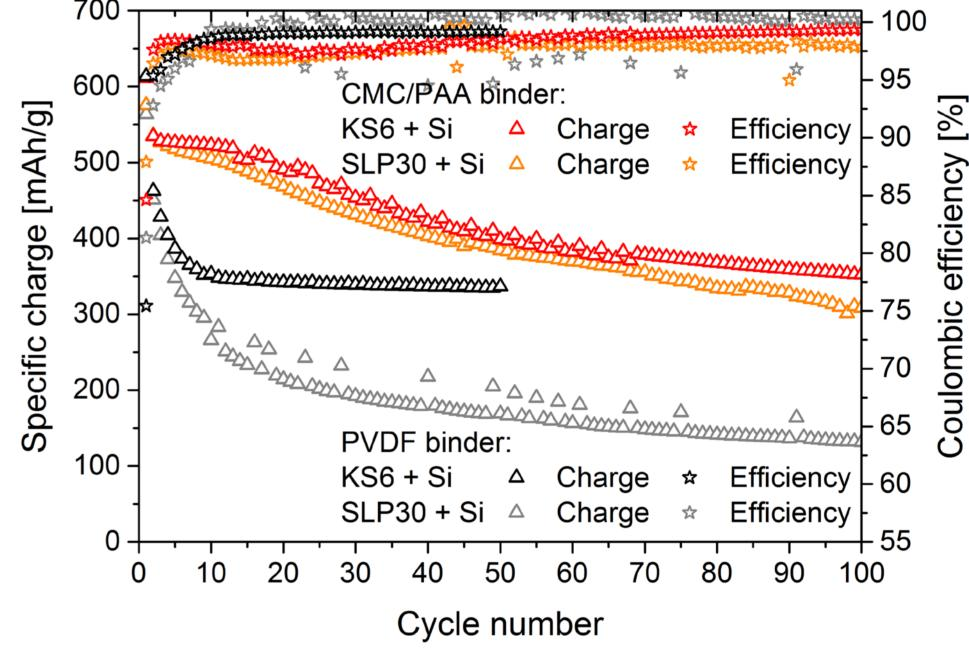
using CMC/PAA: improved cycling stability for both KS6 and SLP30 based electrodes containing Si
