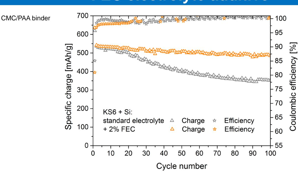
> enhanced cycling stability in presence of fluoroethylene carbonate (FEC)
