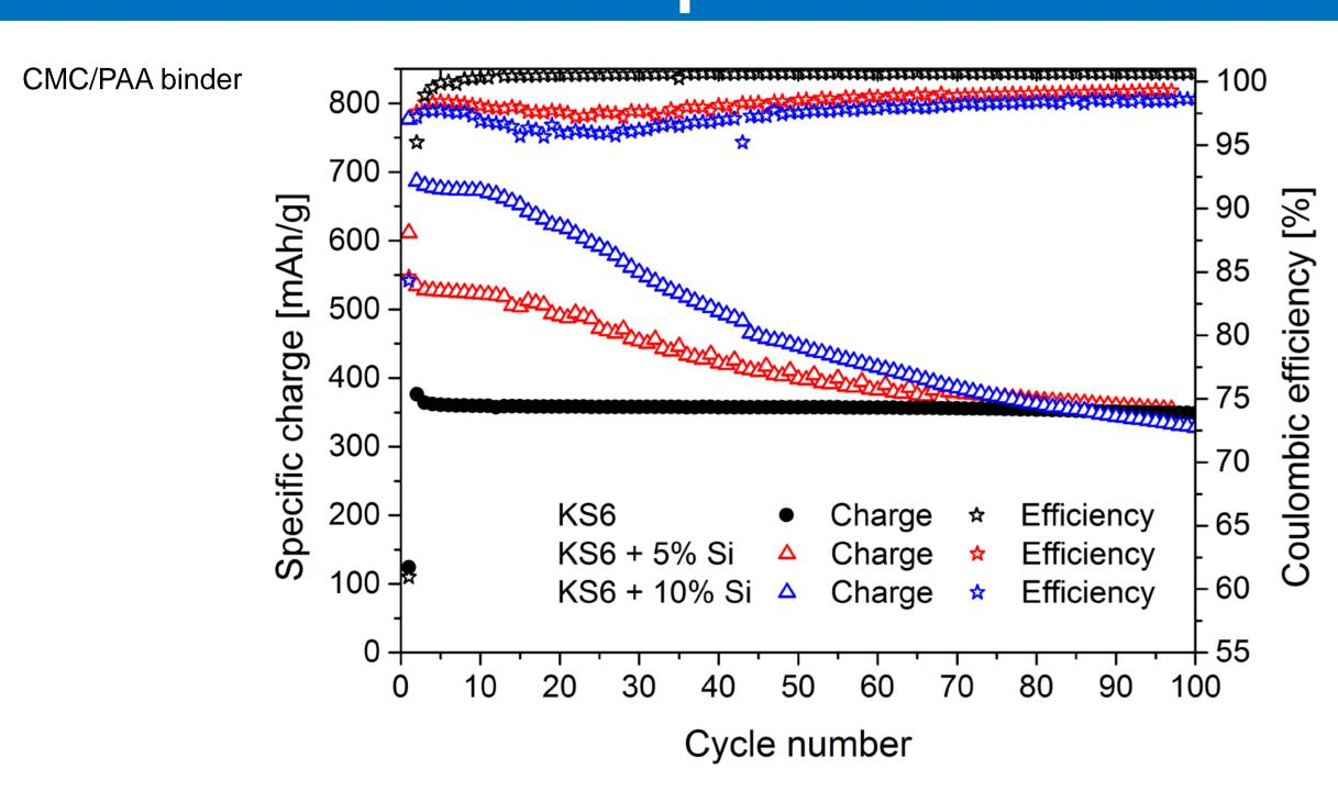
➤ higher specific charge for first cycles with 10 % Si – but stronger fading
