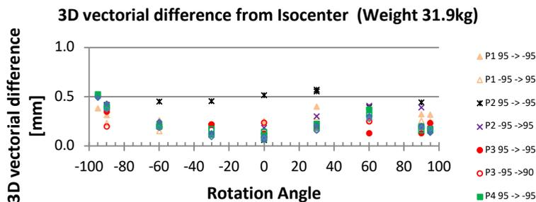
**Figure 1:** Results for patient table isocentric rotations for a weight distribution of 31.9 kg. The rotation range of motion is from -95° to 95°. 95 -> -95 refers to clockwise rotations and -95 -> 95 refers to counter clockwise rotations.
