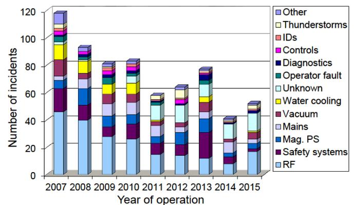
**Figure 4:** Beam outage count per failure category
