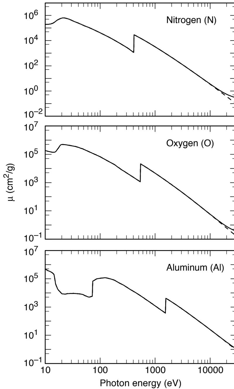
**Fig. 1-5.** Nitrogen, oxygen and aluminium mass absorption coefficients
