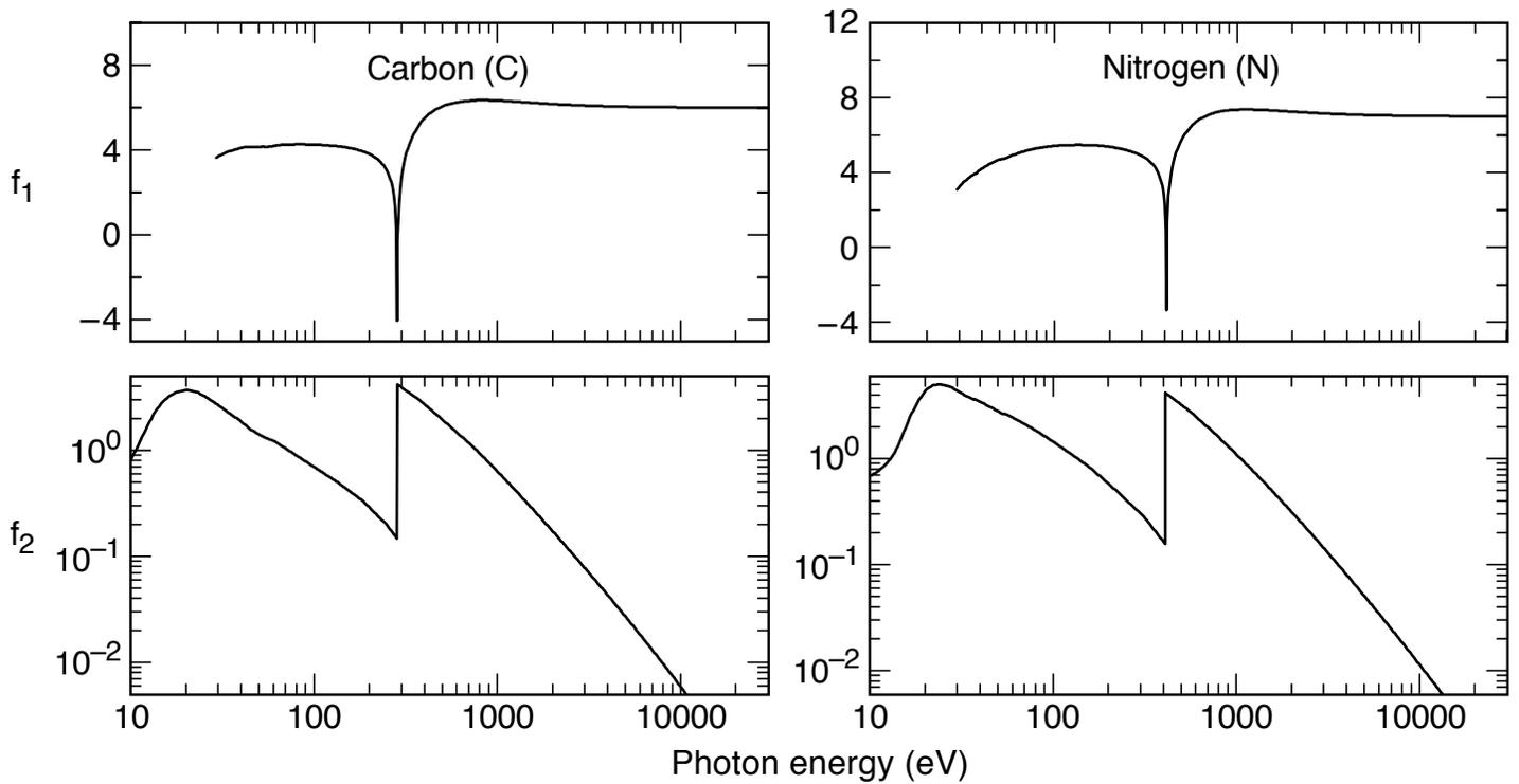
**Fig. 1-6.** Carbon and Nitrogen scattering factors.
