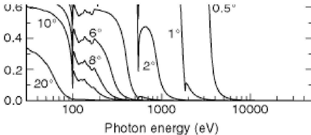
**Fig. 4-4.** *Specular reflectivities of carbon ( $\rho = 2.2 \text{ g/cm}^3$ ), silicon ( $\rho = 2.33 \text{ g/cm}^3$ ), and silicon dioxide ( $\rho = 2.2 \text{ g/cm}^3$ ). The reflectivity is calculated for *s*-polarization at grazing angles of 0.5, 1, 2, 4, 6, 8, 10, and 20 degrees.*
