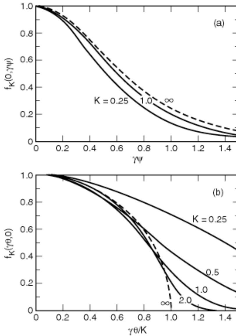
**Fig. 2-7.** The angular function  $f_K$ , for different values of the deflection parameter  $K$ , (a) as a function of the vertical observation angle  $\psi$  when the horizontal observation angle  $\theta = 0$  and (b) as a function of  $\theta$  when  $\psi = 0$ .
