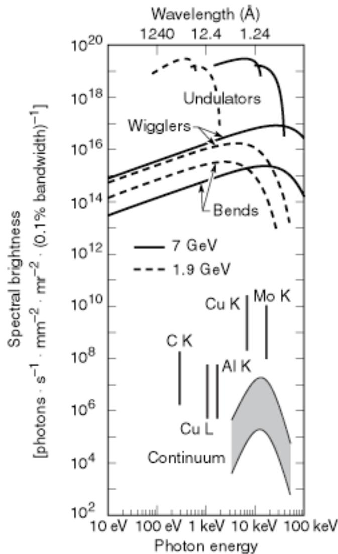
**Fig. 2-9.** Spectral brightness for several synchrotron radiation sources and conventional x-ray sources. The data for conventional x-ray tubes should be taken as rough estimates only, since brightness depends strongly on such
