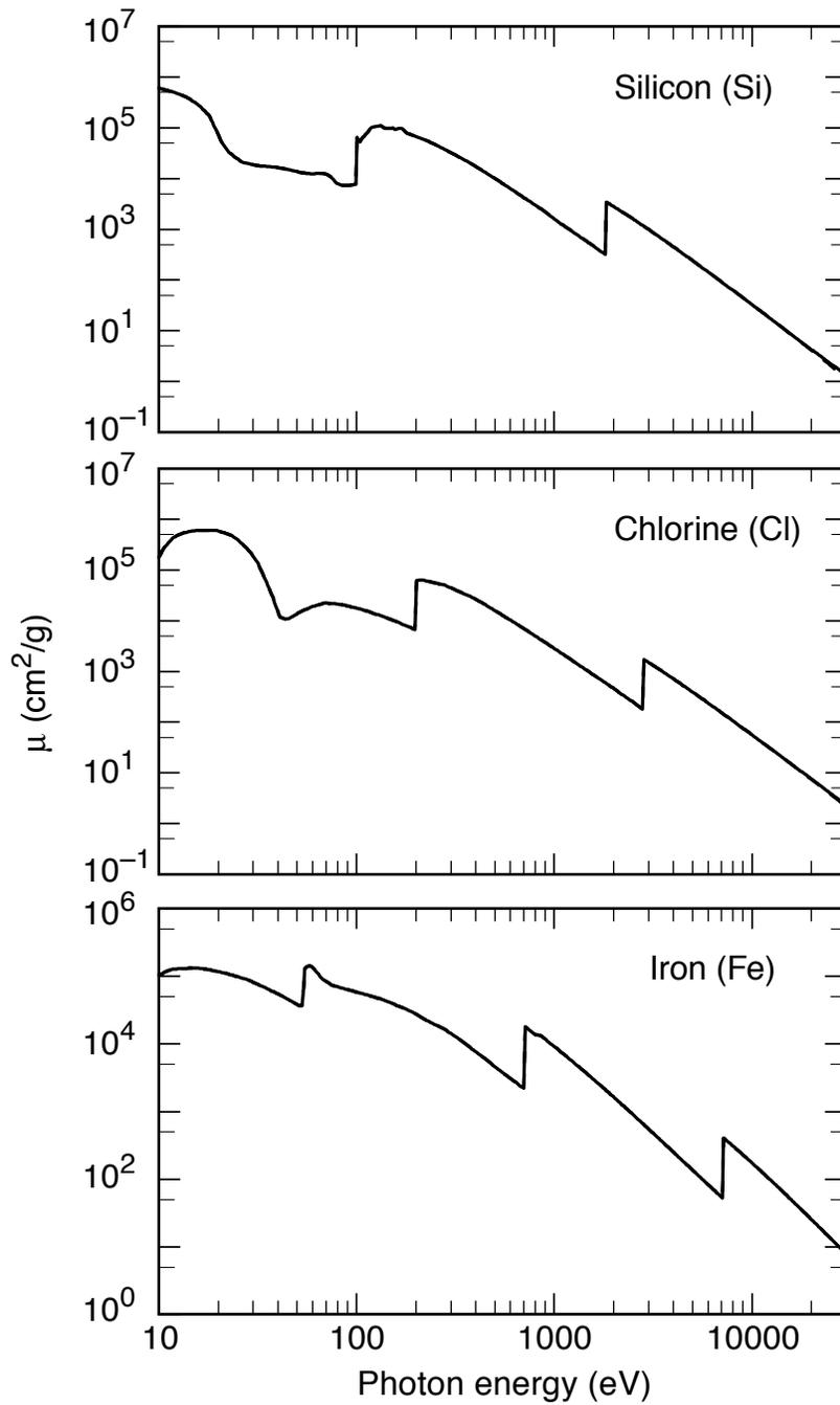
*Fig. 1-5. Silicon, chlorine and iron mass absorption coefficients.*
