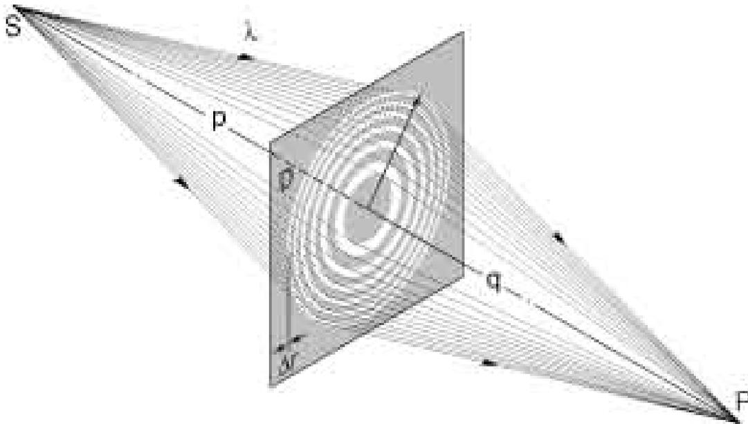
**Fig. 4-9.** A Fresnel zone plate used as a diffractive lens to form an x-ray image of a source point  $S$  in the image plane at  $P$ . The lens is shown as having a diameter  $D$  and outer zone width  $\Delta r$ . The object and image distances are  $p$  and  $q$ , respectively. A full-field image is formed concurrently in this manner. [Courtesy of Cambridge University Press, Ref. 3.]
