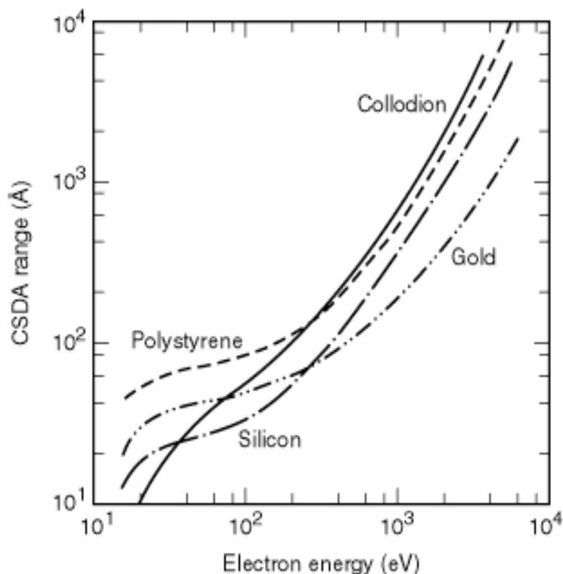
**Fig. 3-3.** Plot of the CSDA range, as a function of energy, for gold and silicon [5] and for polystyrene,  $(C_8H_8)_n$ , with a density of  $1.05 \text{ g/cm}^3$  [2]. The measured electron range in collodion with a density of  $1 \text{ g/cm}^3$  is also plotted [7].
