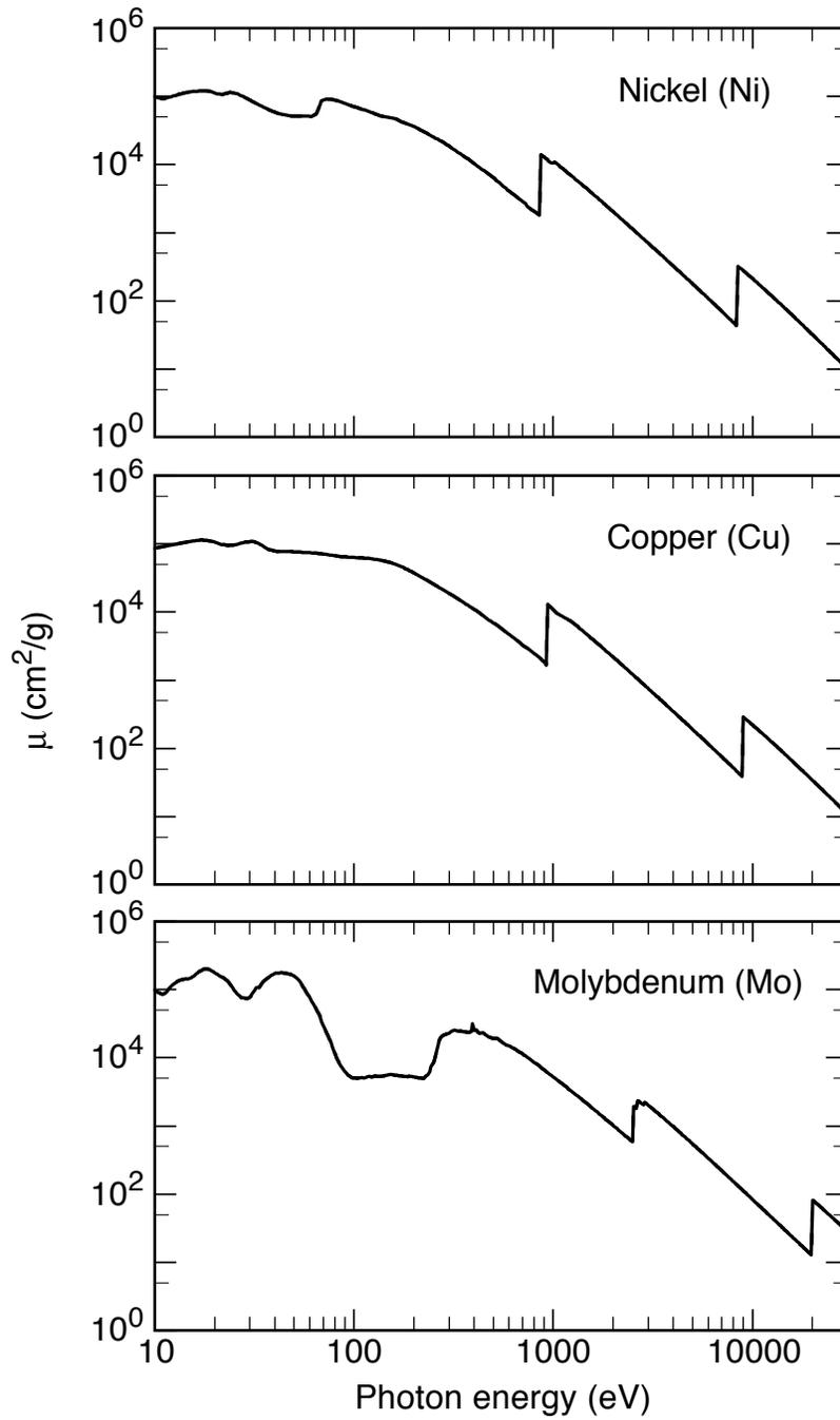
**Fig. 1-5.** *Nickel, copper and molybdenum mass absorption coefficients.*
