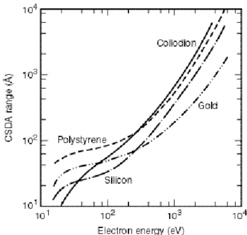
**Fig. 3-3.** Plot of the CSDA range, as a function of energy, for gold and silicon [5] and for polystyrene,  $(C_8H_8)_n$ , with a density of  $1.05 \text{ g/cm}^3$  [2]. The measured electron range in collodion with a density of  $1 \text{ g/cm}^3$  is also plotted [7].
