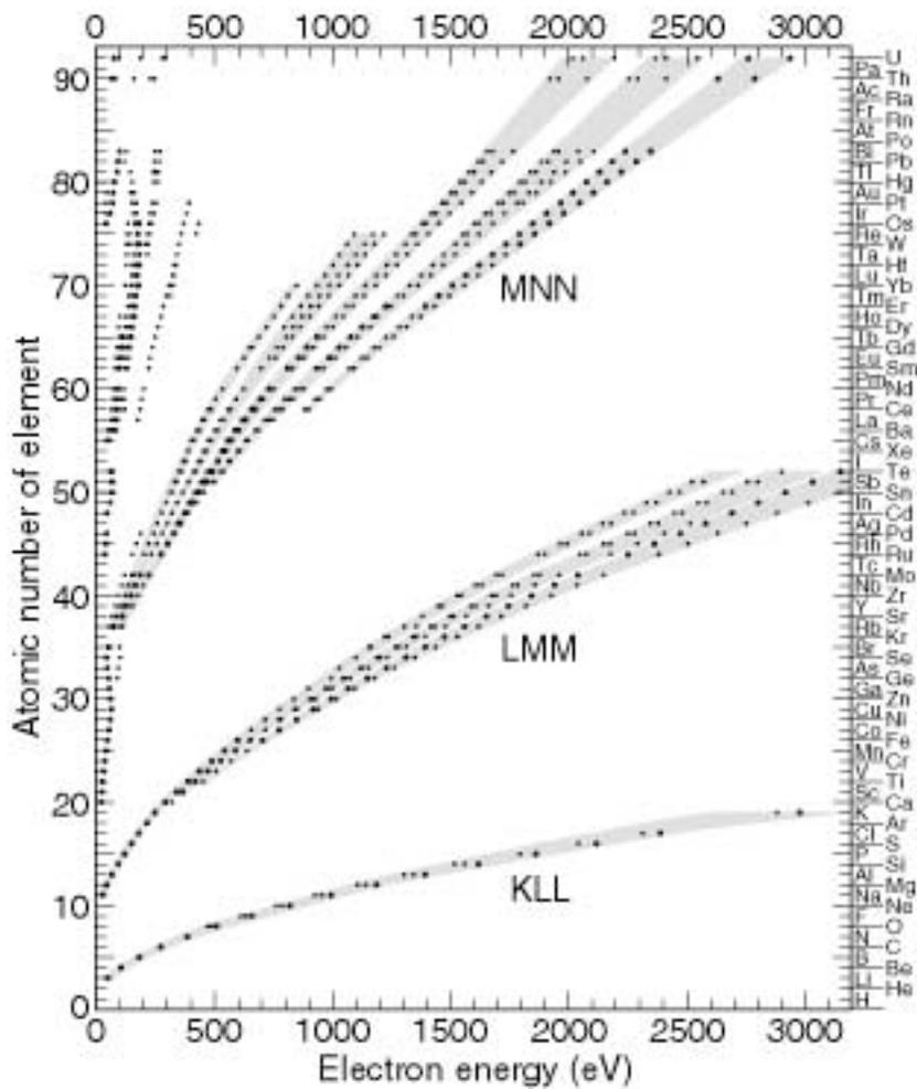
**Fig. 1-3.** Auger electron energies for the elements. Points indicate the electron energies of the principal Auger peaks for each element. The larger points represent the most intense peaks. (Reproduced by permission of Physical Electronics, Inc.)
