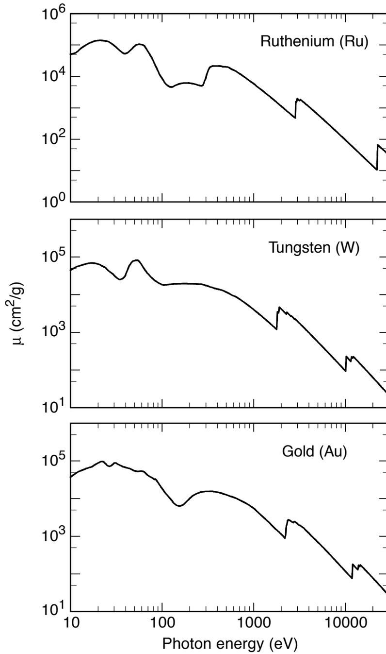
**Fig. 1-5.** Ruthenium, tungsten and gold mass absorption coefficients.
