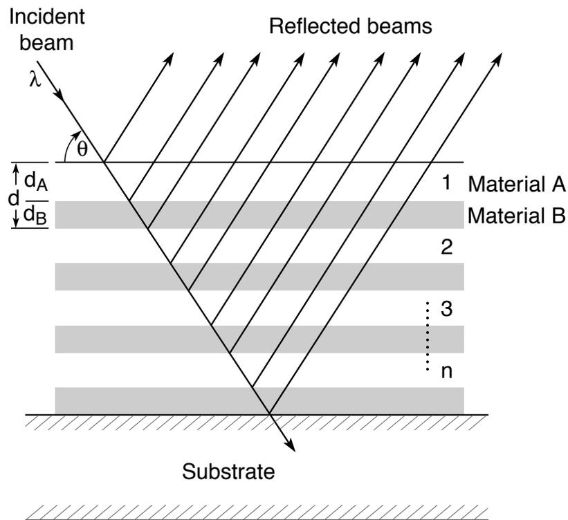
**Fig. 4-1.** Schematic of a multilayer reflector of  $n$  bilayer pairs. The parameters  $\lambda$ ,  $\theta$ , and  $d$  are chosen to satisfy the familiar Bragg equation, but the relative thicknesses of the high- and low- $Z$  materials are also critical in optimizing reflectivity. The total reflectivity is the vector sum of the complex reflection coefficients at each interface, with the different path lengths taken into account.
