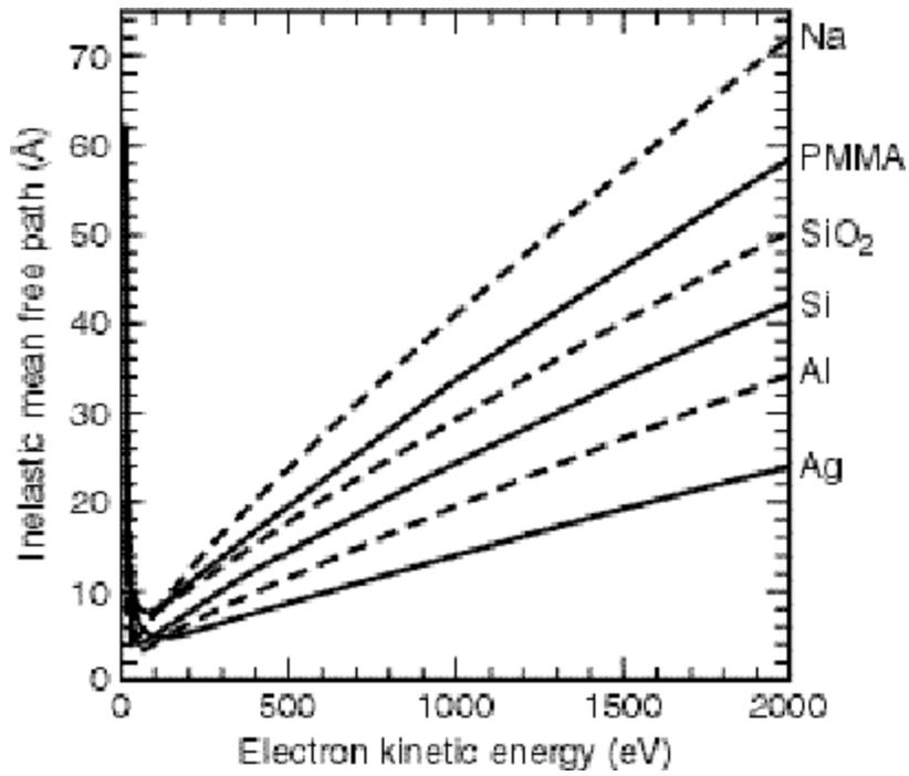
**Fig. 3-4.** Inelastic mean free paths for electron kinetic energies up to 2000 eV, for Ag, Al, Na, PMMA, Si, and SiO<sub>2</sub>.
