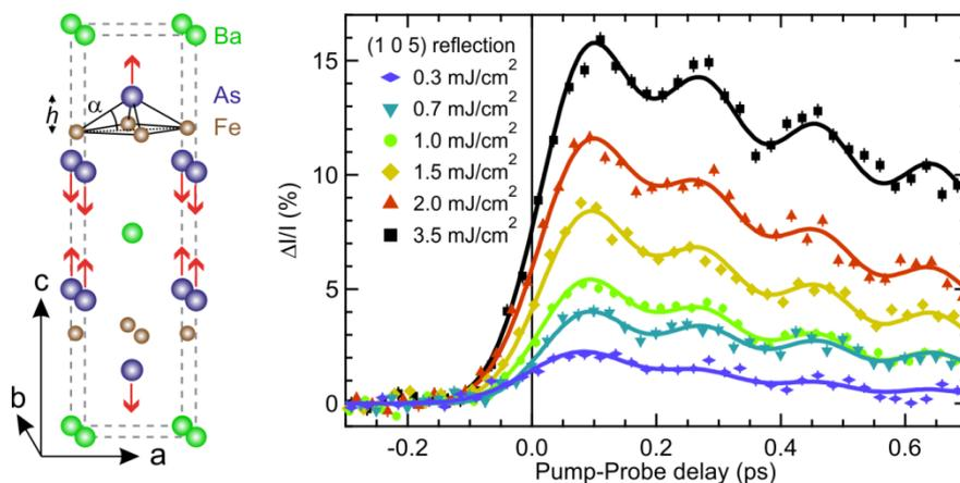
Figure 1. Left: Structure of  $\text{BaFe}_2\text{As}_2$  with the motion pattern of the  $A_{1g}$  phonon mode (red arrows). Right: Pump-induced change of diffraction intensity of the (1 0 5) reflection.
