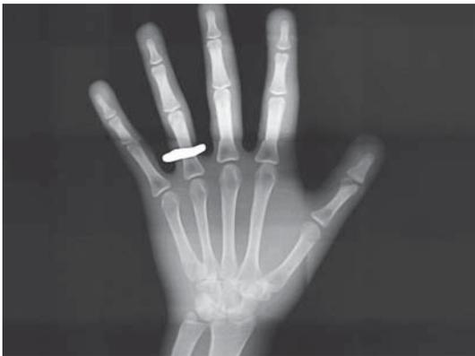
First image of a hand phantom acquired with the GlobalDiagnostiX detector prototype.
