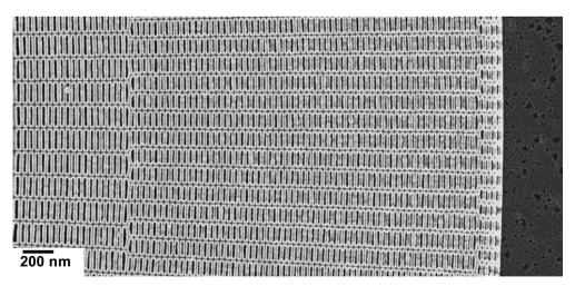
Figure 1: Fresnel zone plate with line-doubled iridium zones of 9 nm line width.
