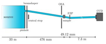
Figure 1: Schematic drawing of a Fourier ptychographic setup at the cSAXS beamline. A 1 mm beamshaper and a 100  $\mu$ m Fresnel zone plate were used as condenser and objective lens of the X-ray microscope respectively. The condenser was illuminated with a coherent beam at 8.7 keV.
