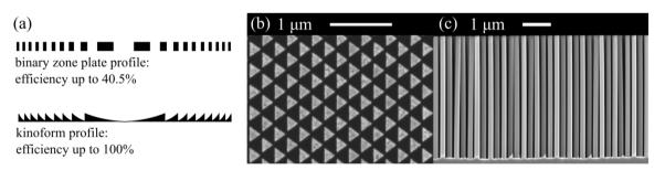
**Fig. 1:** (a): Binary and kinoform phase profiles sketches. (b,c): Scanning electron micrograph of kinoform lenses with 200 nm pitch, showing the (a) top view and the (c) cross section of triangular kinoform elements in silicon.
