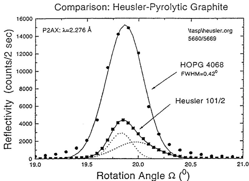
**Fig. 4:** Reflectivity of graphite (002) (circles) and Heusler (111) (squares). The solid and broken lines indicate Gaussian fits. The monochromator size is  $25 \times 50 \text{ mm}^2$ .
