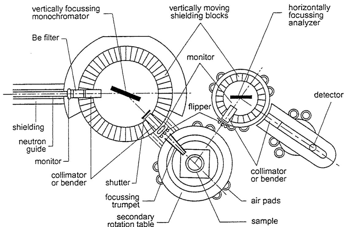
**Fig. 2:** Schematics of the polarized beam, triple-axis spectrometer TASP at SINQ. The instrument moves on air cushions.
