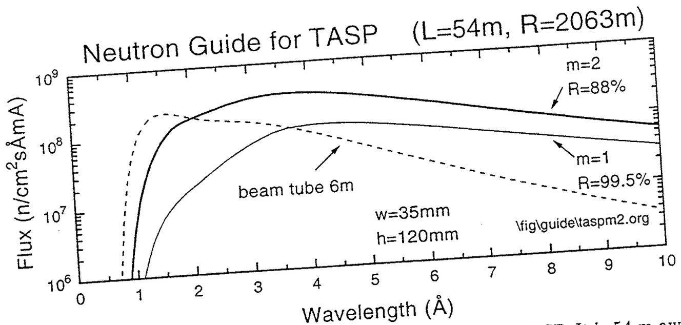
**Fig. 3:** Calculated neutron flux at the monochromator position of TASP. It is 54 m away from the cold source. Also shown is the flux for a "normal" neutron guide, coated with Ni ( $m = 1$ ) and the flux at the end of a 6 m long beam tube.
