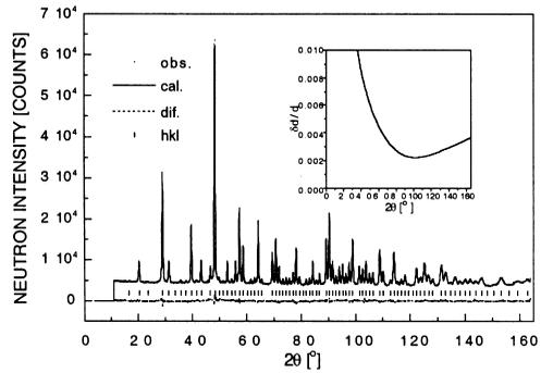
Fig. 5. Observed and calculated neutron diffraction patterns of  $Y_2O_3$  ( $\phi = 8$  mm, lattice parameter  $a = 10.613$  Å, space group  $I a \bar{3}$ ) for  $\lambda = 1.539$  Å,  $2\theta_M = 90^\circ$ , collimations  $\alpha_1 = 12'$ ,  $\alpha_2 \approx 24'$ .
