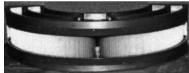
Fig. 4. Radial collimator of HRPT.
