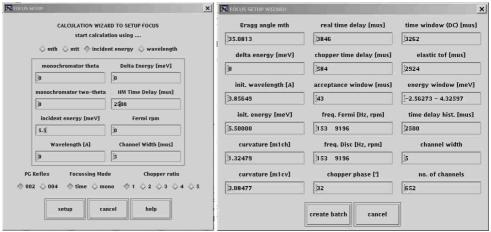
The graphical user interface GUI, distinguishes between *mth* (monochromator theta), *mtt* (monochromator two theta), *incident energy* or incident *wavelength*. Highlight the appropriate button and input the corresponding values into the text field below.
