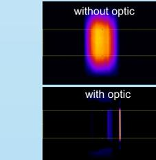
With a prototype adaptive neutron-optical device it was possible to achieve a tiny focal spot on small samples. By adapting the applied force, the y-position of the device and the angle of incidence, the neutrons could be focused in one dimension on a spot size of below 1mm yielding an intensity gain factor of 7.8.
