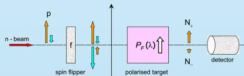
The spin dependence of the neutron proton nuclear interaction can be exploited to build a spin filter operating efficiently over the whole energy range of neutrons from meV to keV. In a test of principle experiment a polarized proton target based on a novel dynamic nuclear polarization (DNP) process has been used to spin filter the white beam at BOA. The system operates at only 0.3 T and 100 K.
