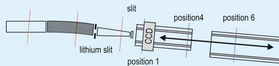
The beam profiles have been measured with different combinations of the lithium slit at the entrance and a slit at the exit of the focusing guide. If the second slit becomes small it acts like a pinhole as was observed in the example below. The McStas simulations reproduce the peak positions well. The intensity mismatch is due to some unknown behavior in the beam path not included in the simulations.
