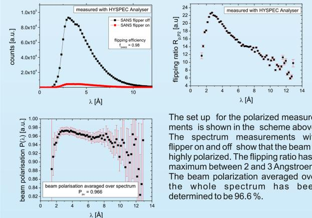
The set up for the polarized measurements is shown in the scheme above. The spectrum measurements with flipper on and off show that the beam is highly polarized. The flipping ratio has a maximum between 2 and 3 Angstrom. The beam polarization averaged over the whole spectrum has been determined to be 96.6 %.
