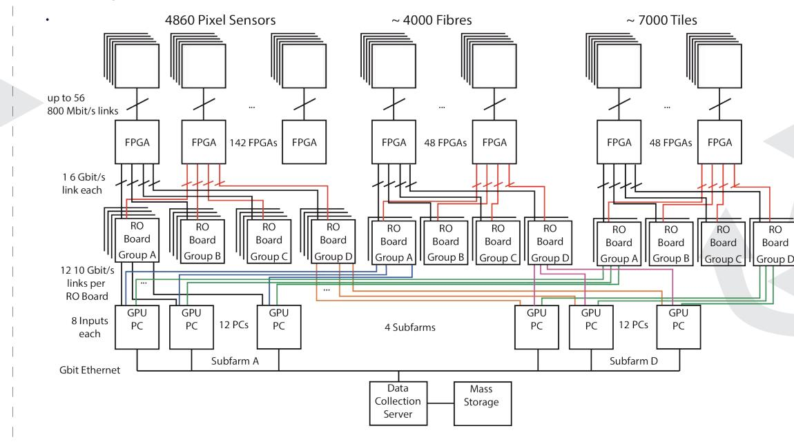
Altera FPGAs are used for **preprocessing** (time sorting and merging) and transmitting the sensor data. Development Kits are used for various tests.
