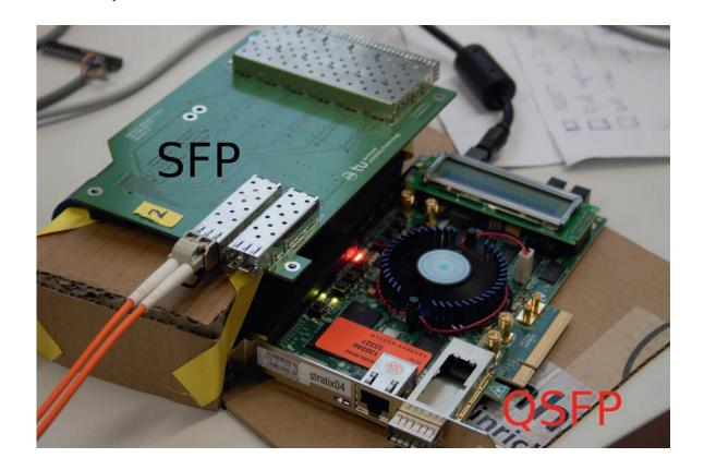
• parity controle on a 80 bit base is needed **6.4 Gbit/s** (BER < 10<sup>-16</sup>) • SFP: • QSFP: **11.3 Gbit/s** (BER < 10<sup>-16</sup>)
