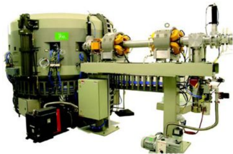
Fig. 2: Cyclotron IBA Cyclone® 18/9, fitted with Vectio® external beam line for advanced research.
