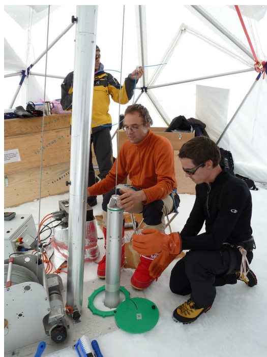
Fig. 1: Ice coring with the thermal drill at Ewigschneefeld.
