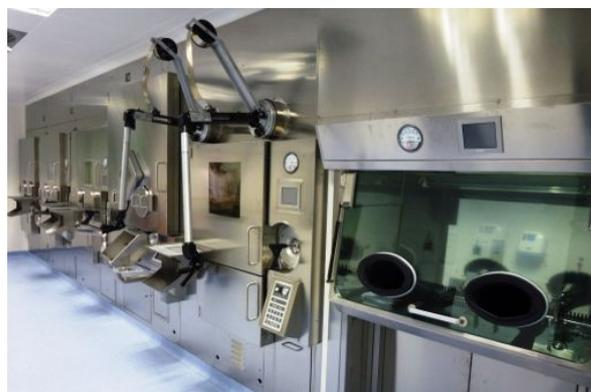
**Fig. 1:** Photograph of the GMP compliant R&D laboratory equipped with hotcells (see text).
