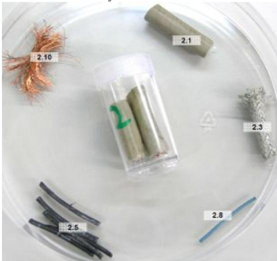
**Fig. 1:** Photo of the cable number 2 (middle) and its individual components (around).
