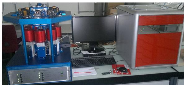
**Fig. 2:** The automated graphitisation equipment (AGE) for routine production of solid AMS targets.
