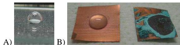
**Fig. 2:** (A) A drop of water placed on a Teflon-AF covered glass plate; (B) A drop of  $\text{HNO}_3$  conc. placed on Teflon-AF covered (left) and uncovered (right) copper foils
