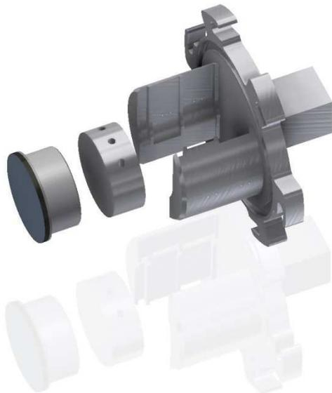
**Fig. 1:** New RbCl target assembly. (Exploded View)
