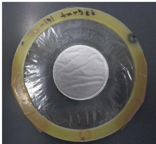
**Fig. 2:** Final  $^{171}\text{Tm}$  target delivered to the CERN n\_TOF community.
