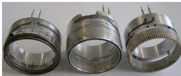
**Fig. 1:** Melting head with *hotspring®* coil heater of 100 mm outer diameter. Left: open heater, middle: simple aluminum heat spreader, right: aluminum crown with heatspreader fins.
