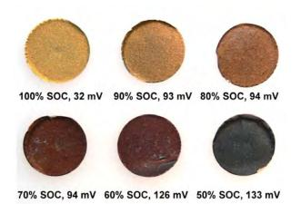
Figure 1. Graphite electrodes harvested from coin cells after intercalation of different amounts of lithium.
