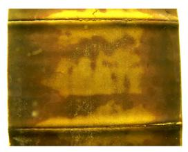
Figure 3. Anode of a commercial high-power cell after 1500 cycles at 6C rate.
