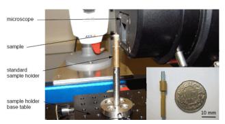
**Figure 1.** Endstation of X02DA TOMCAT beamline with sample holder, scintillator and CCD camera. The inset shows the specially designed sample holder.
