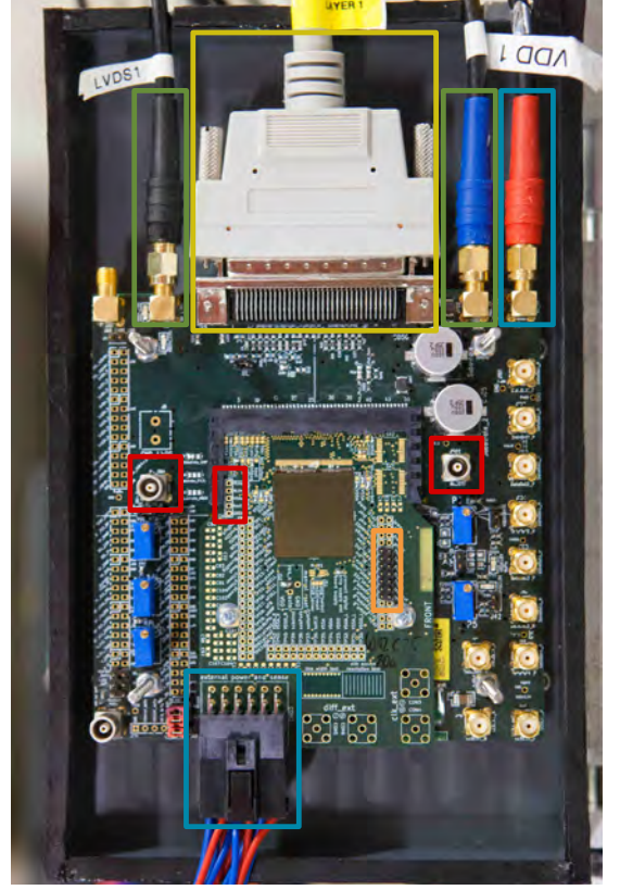
(b) Bottom half-shell of the cooling box with MuDAQ Motherboard and an insert PCB carrying a MuPix10 . Features are highlighted by colored frames: orange indicates TestOut , red marks the connection points for AmpOut , HitBus , and Injection . blue shows the HV (SMA) and low voltage ( Molex ® ) connections for sensor biasing, while green (for MuPix10 ) is exclusively used to power the MuDAQ Motherboard. yellow frames the SCSI-3 connection to the HSMC adapter card.
