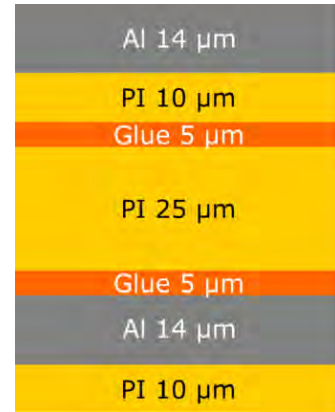
(b) Layer stack of a HDI-flex consisting of alternating layers of aluminium, polyimide and glue. Taken from [78, p. 17, fig. 7.11].
