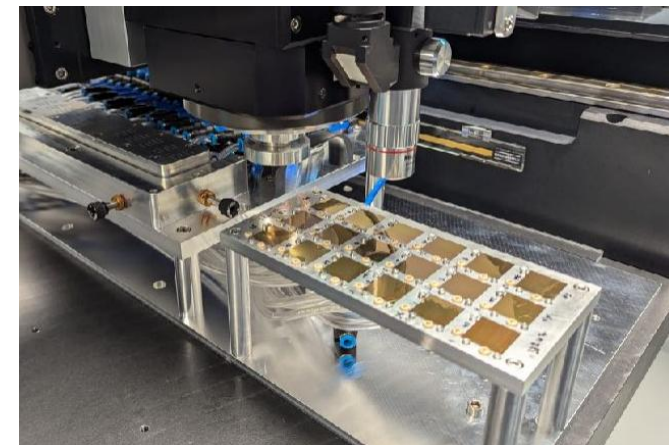
Robotic gantry for chip placement
