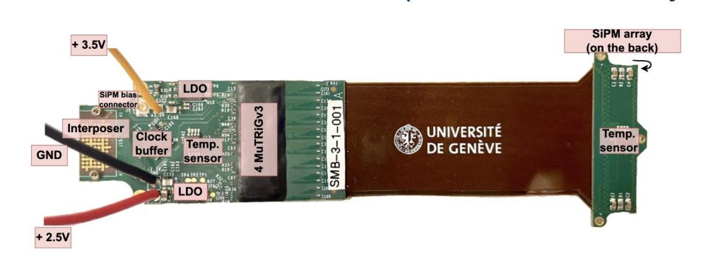
Each ribbon coupled at both ends to Hamamatsu S13552-HRQ SiPM arrays (128 ch, 250 $\mu m$  pitch,  $R_q=500~k\Omega$ )
