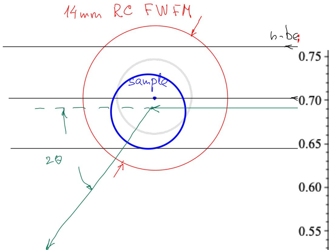
8mm dia sample shifted by 4mm in direction of  $2\theta=90\text{deg}$
