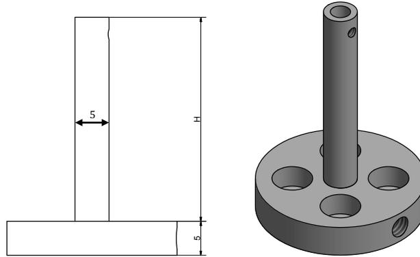
This sample holder is for pin diameter of 3.15mm
