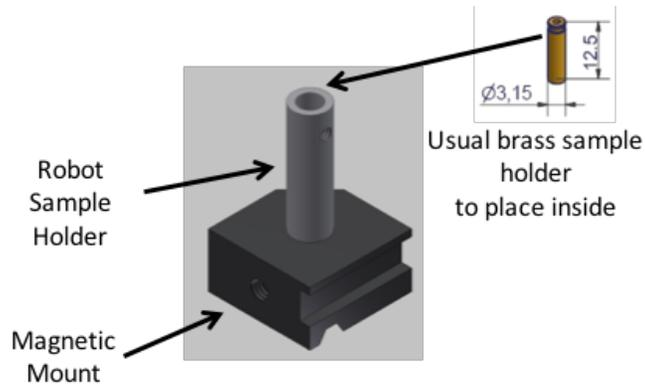
Note that the pin is screwed on the side of the robot sample holder. Ideally the pin or the sample should have a diameter of 3,15mm or smaller but not larger.
