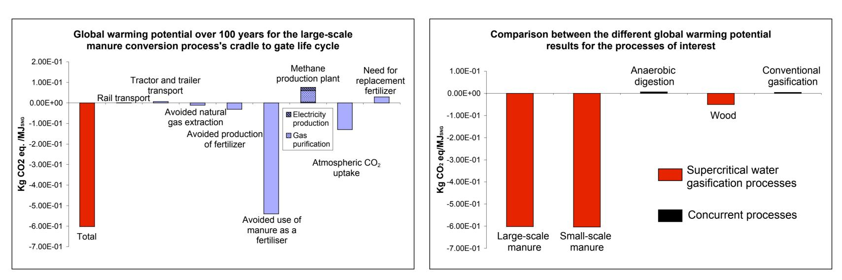
The global warming potential is calculated for the modeled scenarios and benchmarked toward concurrent processes (anaerobic digestion of manure and conventional wood gasification)
