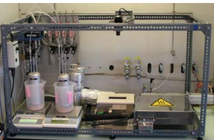
Lab setup of channel reactor with the feed system (left side of picture), channel reactor (in the middle of the picture), heating box for sampling capillary (right side of picture) and the infrared camera (top section of the picture)
