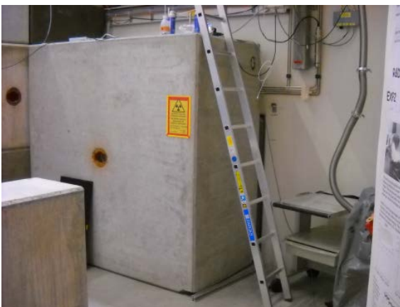
Fig.12: Concrete block shielding the spallation target between area West-1 and West-2. The slits on the wall are a source of background radiation for the experiments.
