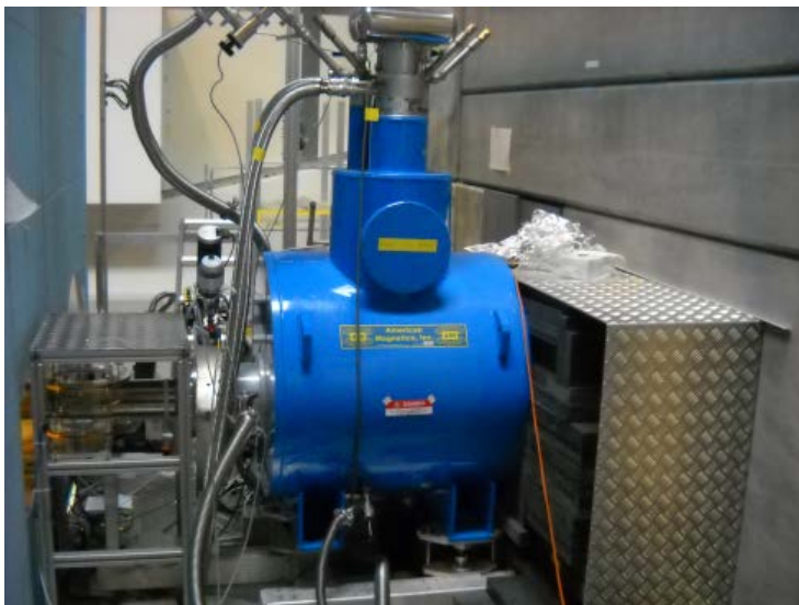
Fig.16: beam port area south - the 5 Tesla super-conducting magnet in blue
