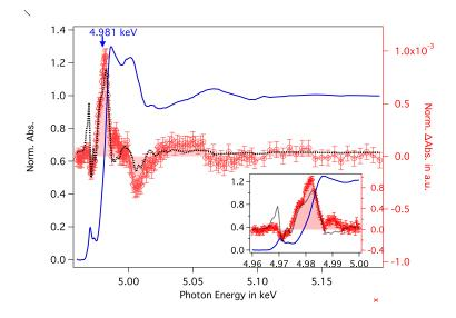
Fig. 1: The ground state Ti K -edge x-ray absorption spectrum (blue line) of TiO<sub>2</sub> nanoparticles together with the transient XAS difference spectrum (red circles) measured 100 ps after excitation. Inset shows zoom of pre-edge peaks.
