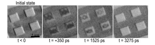
Figure 1: Sequence of TR XMCD images of GdFeCo taken at Fe L3 edge. The images show the magnetic configurations in 5  $\mu$ m squares imaged before the excitation with a linearly polarized laser pulse and at different delays after the laser excitation.
