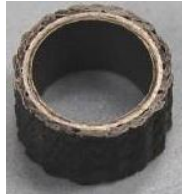
Piece of potential cladding tube (SiC/SiC with Ta)
