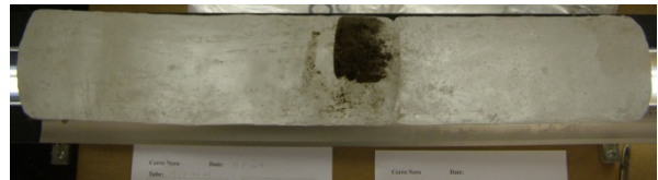
Fig. 1. Photo of the topmost core from Cerro Negro glacier showing transparent ice with few air bubbles and a ca. 8 cm thick dark layer at ca. 40-48 cm depth.
