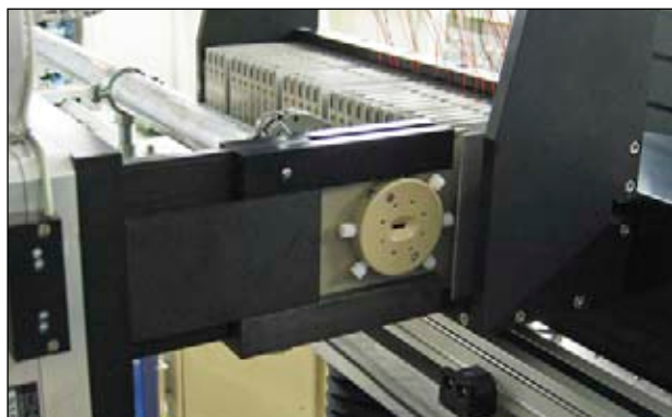
Figure 2: Sample changer developed at PSI for the MS beamline of the SLS.
