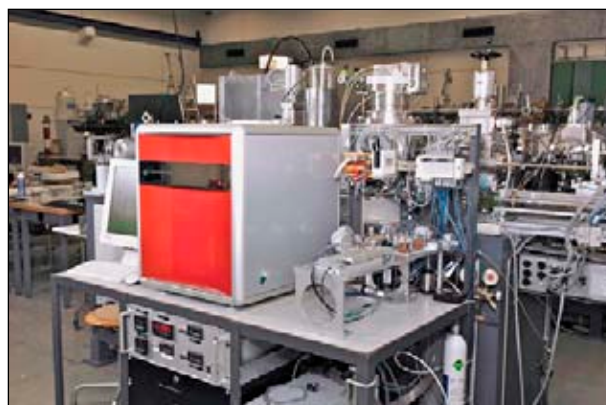
Figure 1: Miniaturized gas-handling system for the direct injection of a few micro-liters of \text{CO}_2 gas into the MICADAS for radiocarbon dating. The heart of the system is a gas-tight syringe from which the gas is pressed into the ion source via a capillary.
