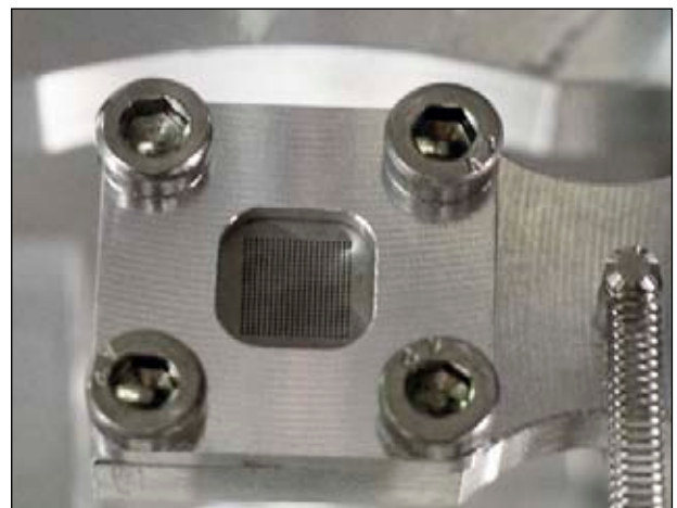
Figure 1: The tungsten mask (“pepper-pot”) intercepting the electron beam...
