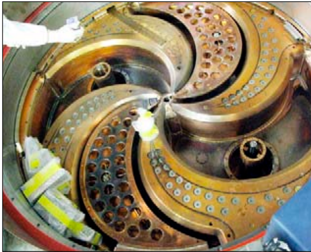
Figure 5: View on the lower pole of the cyclotron before assembly of the Dees on the two new stems.
