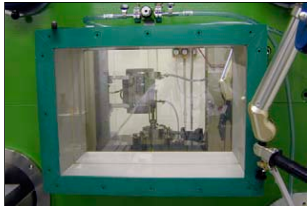
Figure 4: Remotely operated mechanical test machine behind its shielding.
