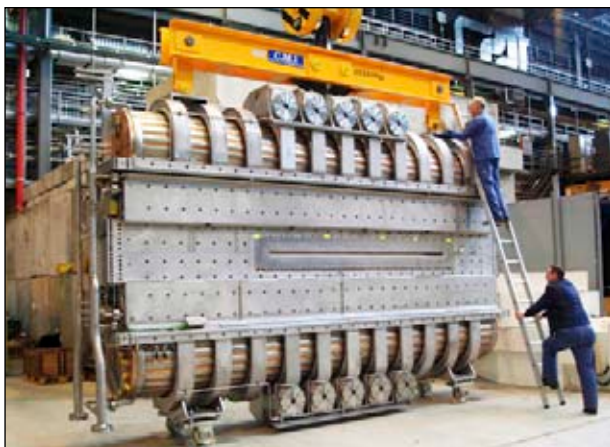
Figure 1: One of the four new copper cavities inserted into the Ring Cyclotron.
