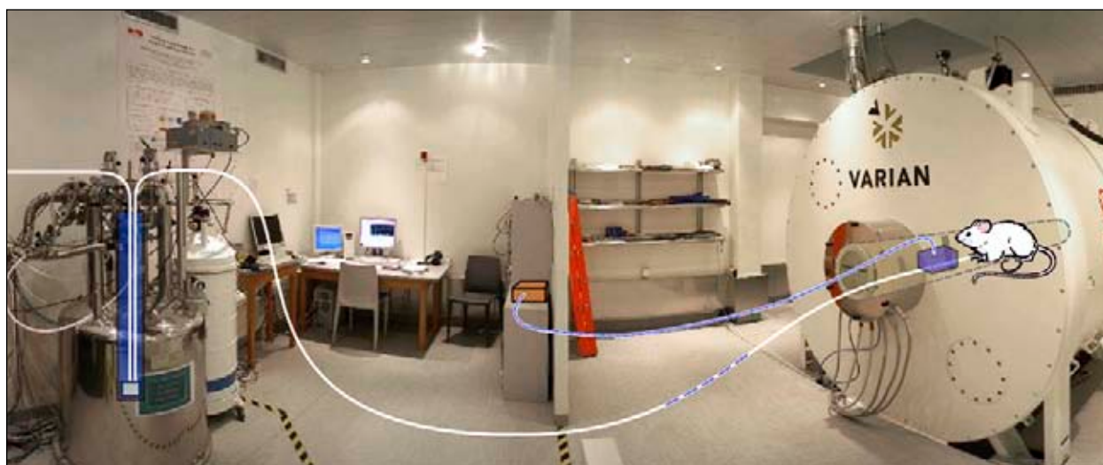
Figure 1: Dissolution DNP machine (left) connected to the 9.4 T rodent scanner (right) installed at the CIBM Lausanne. The sample is polarized in the solid state at around 1 K at 3.35 T and subsequently rapidly dissolved and blown via a thin tube to an injection pump delivering the polarized room temperature solution to the animal in the imager [7].
