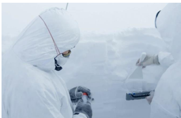
Fig. 1: High-Alpine snow is very sensitive to contamination due to the low concentrations of atmospheric TEs. Therefore, special precautions, such as wearing clean room overalls, facemasks, and ultra-clean plastic gloves, were taken during the snow pit samplings.
