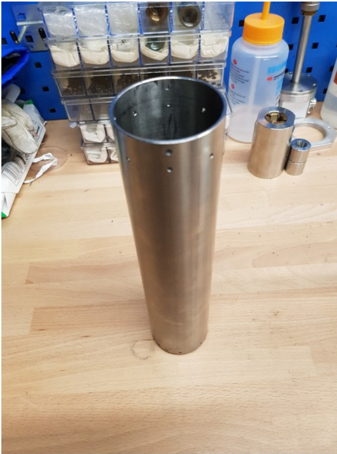
Protective Cylinder for ACS measurements
