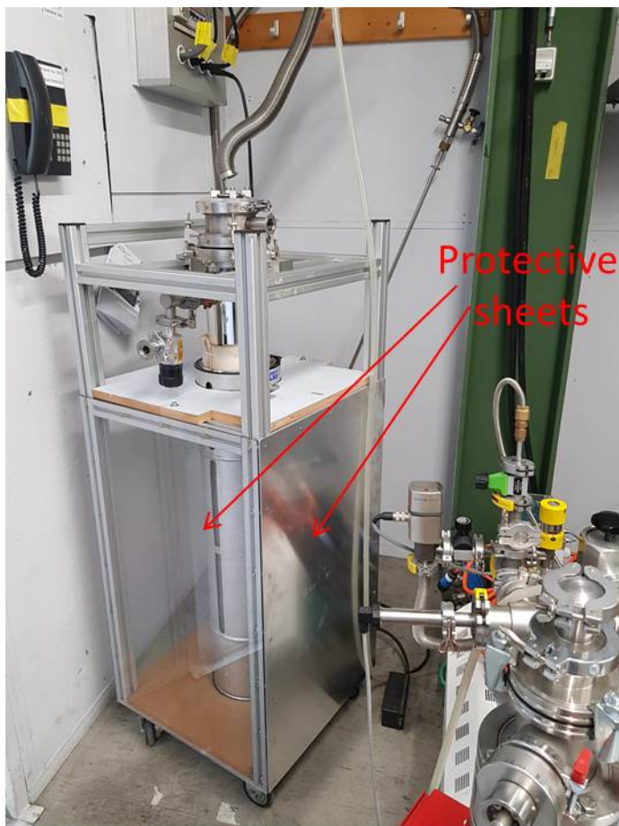
ACS glass cryostat with protective sheets
