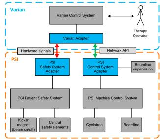
Principle for the Varian/PSI Control and Safety System Integration. Varian's and PSI's control system are left untouched. Dedicated adapters serve as interface between the two worlds. Control signals are passed over the network whereas safety critical signals are connected by hardware lines.
