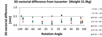
Figure 1: Results for patient table isocentric rotations for a weight distribution of 31.9 kg. The rotation range of motion is from -95° to 95°. 95 -> -95 refers to clockwise rotations and -95 -> 95 refers to counter clockwise rotations.
