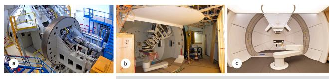
Installation of Gantry 3: a) shows the end of the beamline, the coupling point to the Gantry and the Gantry corpus from behind in the machine room; b) shows the (future) treatment room without any wall cladding; c) shows the final treatment room with the patient couch in front and the beam head (called nozzle) on top, from which the proton beam emerges.
