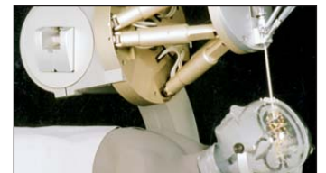
Custom Hexapod designed for neurosurgery Photo: IPA
