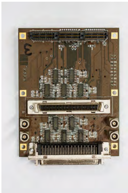
(A) FPGA side LVDS card.
