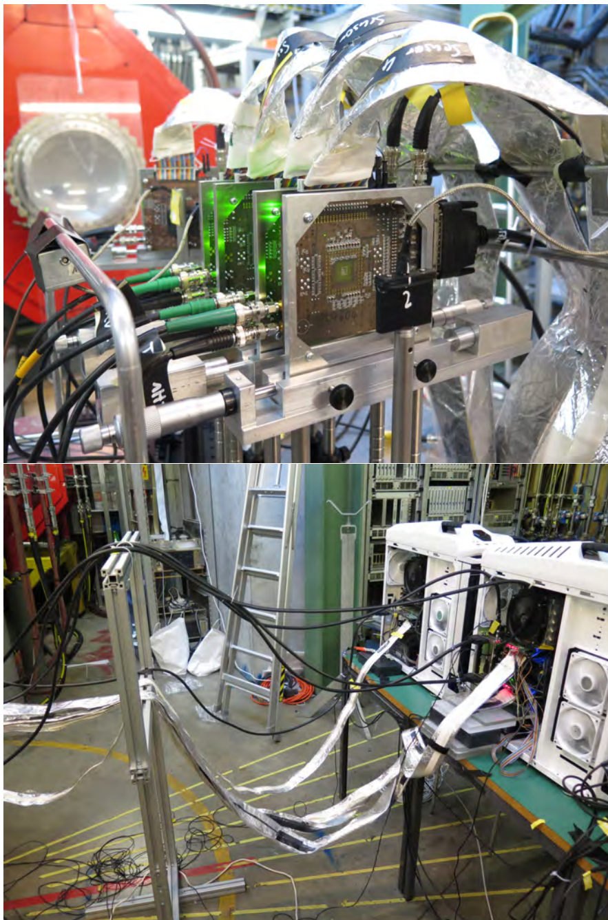
FIGURE 9.1: Pictures of the PSI setup: The top picture shows a close view of the setup from the backside. The red magnet in the back is the last quadrupole from the beamline with the beam window, secured by a plastic plate. The bottom picture shows the cabling to the readout computer. The front computer is the telescope readout PC, the back one is used for the single MuPix setup.
