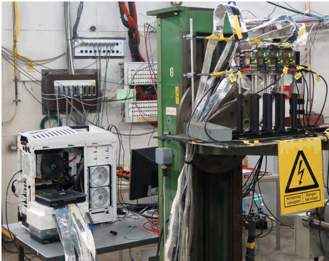
FIGURE 8.3: The DESY testbeam setup: On the top right, the telescope, mounted on a movable stage, provided by the DESY testbeam group. The telescope is connected to the RO computer via 4 m long shielded ribbon cables.
