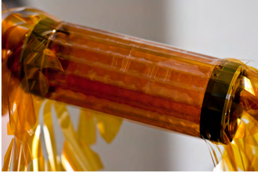
Figure 2.5: First mechanical prototype of the Kapton support structure for the inner two layers (length: 12 cm).
