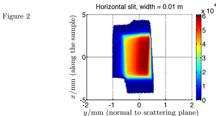
Figure 2 shows the intensity map  $I(x, y)$  at the sample position for a diaphragm opening of 10 mm in  $y$  direction, i.e. normal to the scattering plane, and 50 mm in  $x$  direction, i.e. along the sample surface. One can see that the intensity for  $y < 0$  is smeared out, which means a reduced intensity on the sample, and illumination of the environment.
