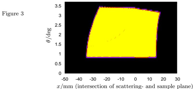
Figure 3 shows the analytically obtained  $I(x, \theta)$  map at the sample position. The footprint is only slightly larger than the horizontal distance of the first slits of 50 mm and the divergence is almost homogeneous over that length.
