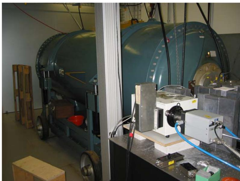
**Figure 2-15.** 2 MeV Febetron 705 accelerator at ETH Zürich, with detection equipment.
