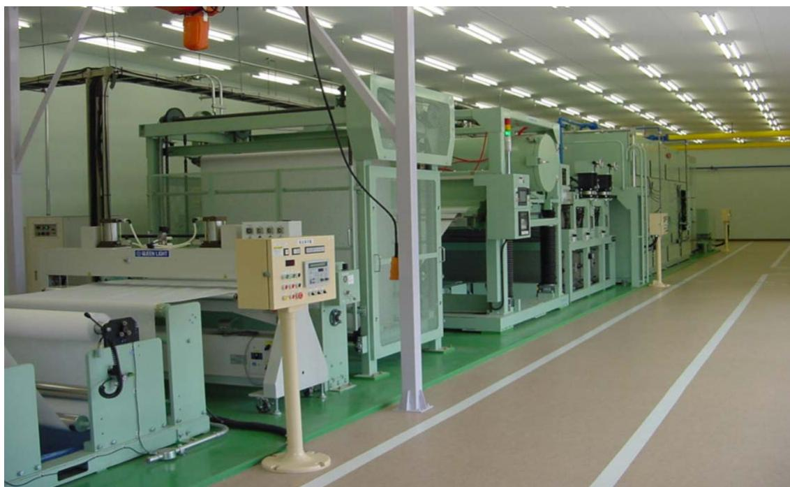
**Figure 0-4.** Reel-to-reel process line for the preparation of functionalized non-woven fabric by pre-irradiation induced grafting [53].
