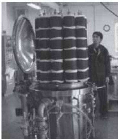
**Figure 0-5.** Batch-mode operated pilot-scale reactor for the manufacture of Cs-adsorptive fiber material [66].
