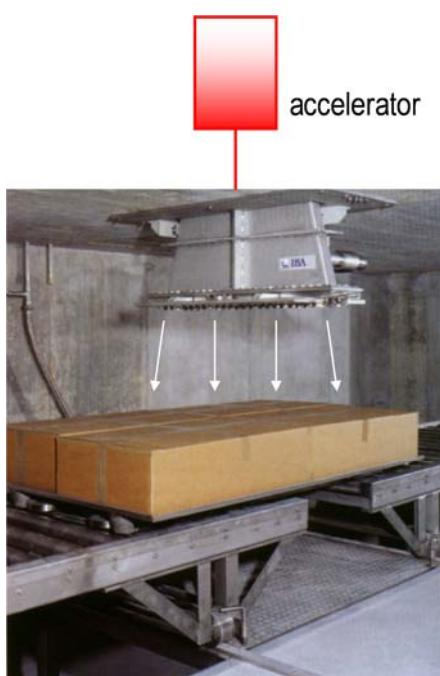
**Figure 2-2.** Electron-beam irradiation of goods conveyed under the scan-horn of an electron accelerator. Typical electron energy is in the MeV range (photo: Leoni Studer AG, Däniken SO, Switzerland).
