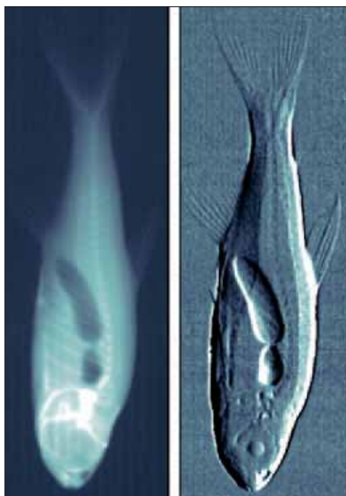
Conventional X-ray image (left); innovative phase contrast X-ray image (right).
