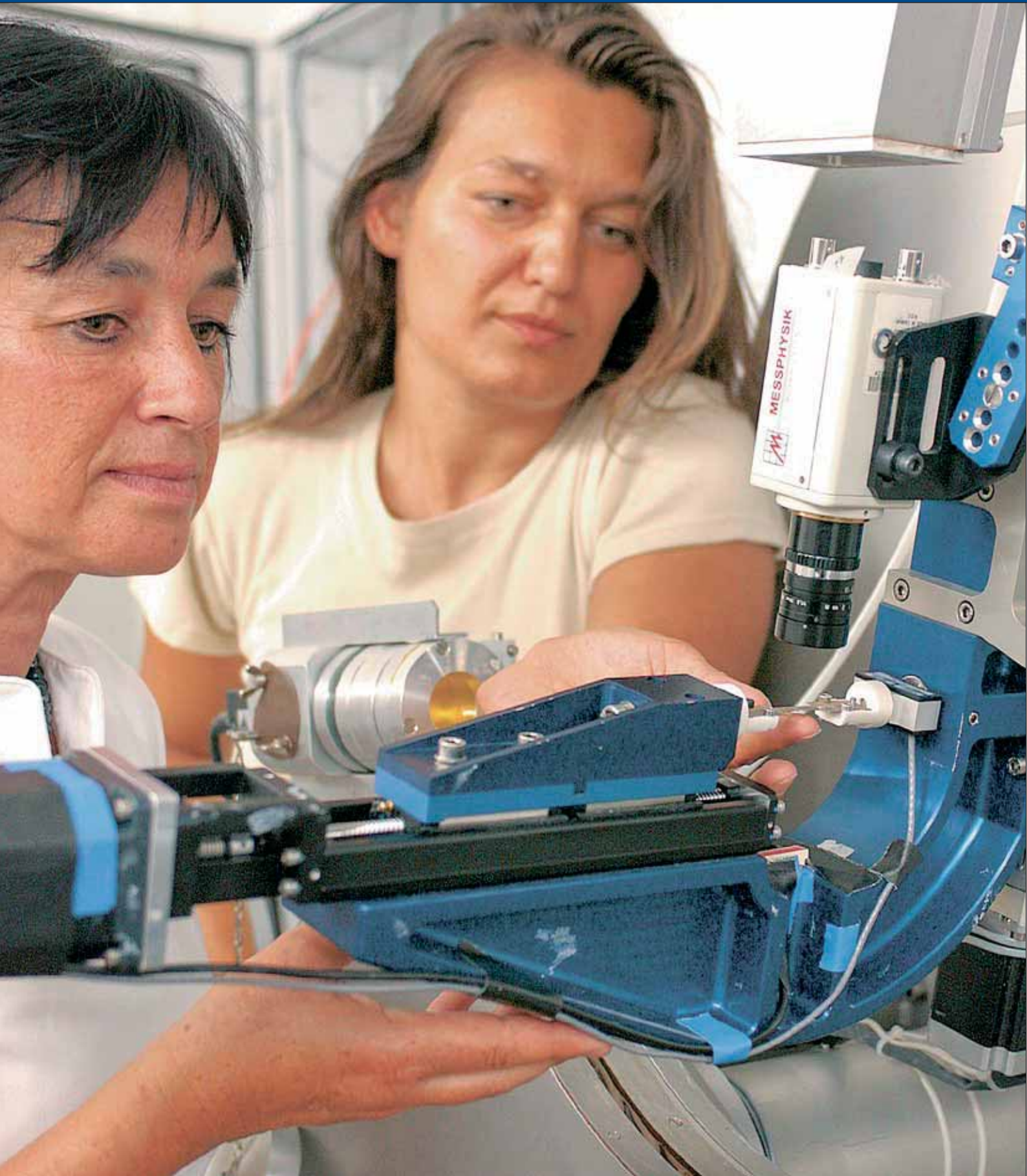
Microcrystals in the focussed X-ray light: researchers fit a sample in the tensile testing machine at the SLS.
