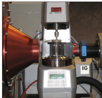
Figure 3: Installation of a standard rheometer on the SANS-1 instrument to study the molecular structure and the rheological properties of a liquid.
