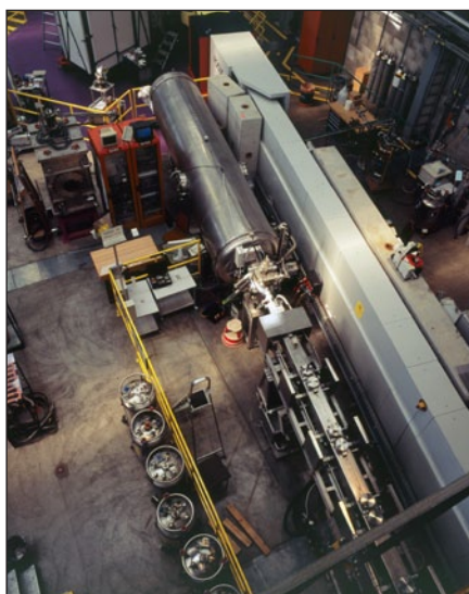
Figure 1: Small-Angle Neutron Scattering instrument (SANS-2) at the Spallation Neutron Source SINQ.
